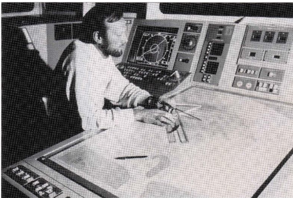
Fig. 6.12 Integration of the predictor with the ship's bridge
