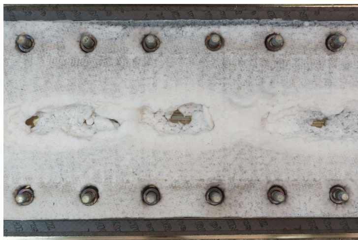
Figure 4.14: Distributed insulation damage, photograph taken from the flow side with the liner removed.
