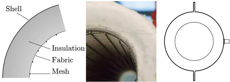
Figure 3.1: Schematic representation of a portion of the sample cross-section with components indicated (left), sample 18-1H-1 before adhesion of the connectors (middle), and schematic representation of a sample during testing with the shell flanges vertical and a gas thermocouple mount on one side (right).
