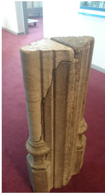
Fitting of first cast, the seam caused by the smoothing of the edges is visible.
