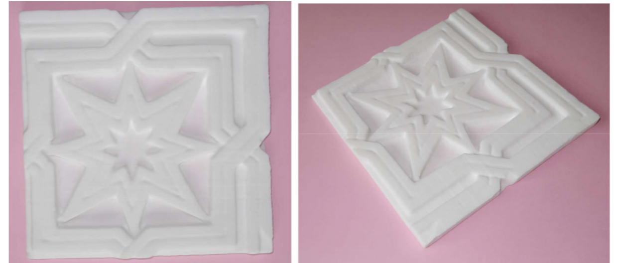
Figure 22. SLS Printing Result. Source: Adrian Gheorghiu
