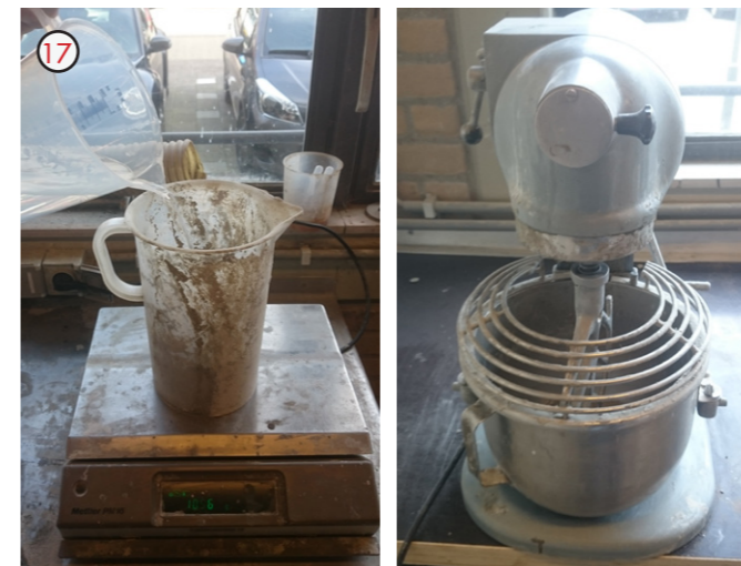
17. The first cement sample was casted with a water-cement (i.tech Ultracem 52.5) ratio of 0.5 and the addition of white pigment (Titanium Dioxide) to lighten the color of the cement.
