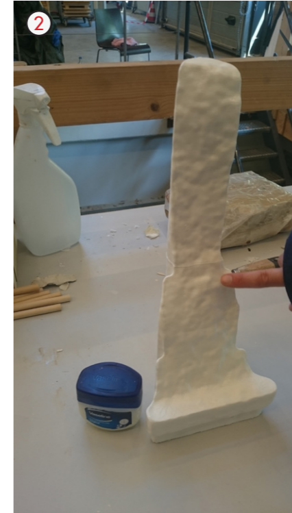
2. A thin layer of Vaseline was applied to all the exposed surfaces as a release agent against the silicone. This also ensures the smooth removal of the pattern from the mold.
