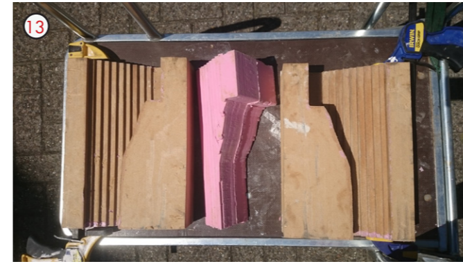
13. The setup was disassembled for inspection after the silicone had cured. In this instance, the inner surface of the mold reinforcement had been contoured to save time but that caused difficulties during disassembly, despite the use of a release agent. Therefore, it is recommended to mill a smooth surface or to use a different material.
