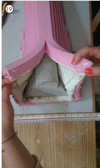
19. The sample was removed after curing for 72 hours. A slight incision had to be made on the mold to extract the cast, the incision would leave minimum marks on any subsequent castings due to the cohesive properties of silicone.
