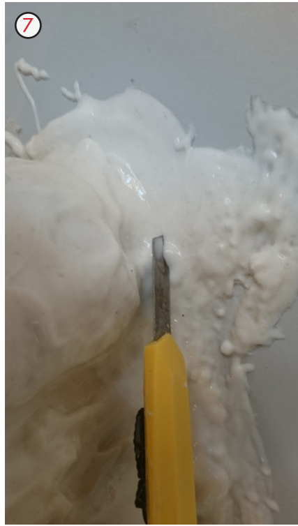
7. The silicone overflow was sliced off using a paper cutting knife to ensure that there is room for a layer for clay to hold the pattern down.
