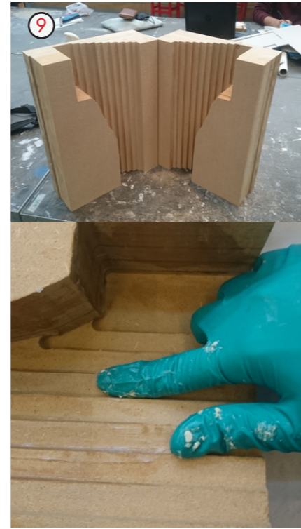
9. An MDF mold reinforcement was CNC milled with an average offset of 2 cm to aid in the pouring of the secondary silicone layer. This MDF container would also help strengthen the mold to prevent any deformations during the casting process.
