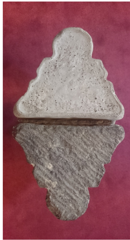
Top of the first column segment with the first cast, displaying the mirroring of the geometry. Small bubbles that escaped from the inside of the cast are also visible.
