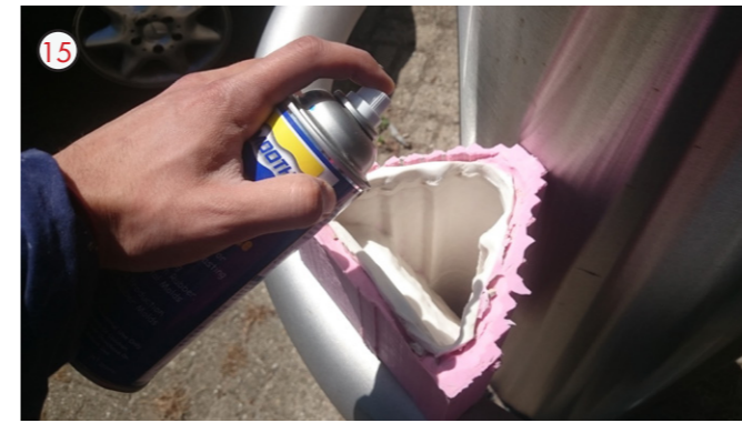
15. A layer of Smooth On Universal Mold Release was applied and left to dry overnight. Another layer was applied 15 minutes before the casting process as instructed by the manufacturers.
