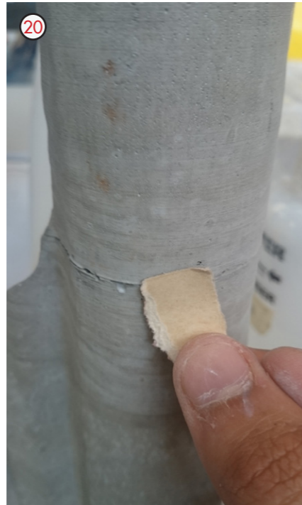
20. The transferred markings from the PLA pattern were then sanded away from the casted material using a medium grit sandpaper.
