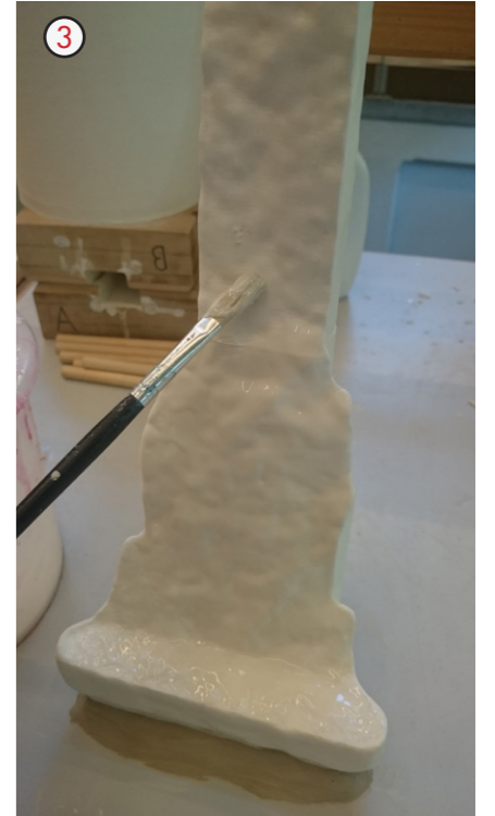
3. The 'pattern' was held down using wet clay and the first layer of silicone (using Mold Max Stroke Part B) was applied to the surface.
