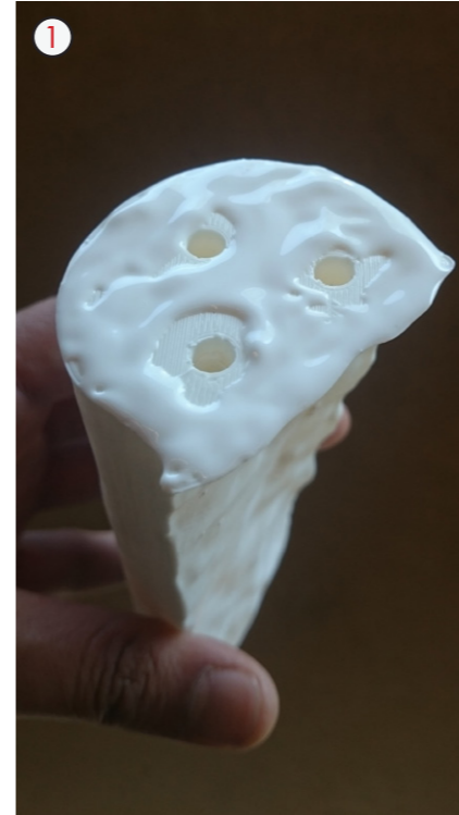
1. Although the two components fit together readily, PVA white glue was still used as a temporary measure in case the silicone leaked inside the cavity between the two pieces.
