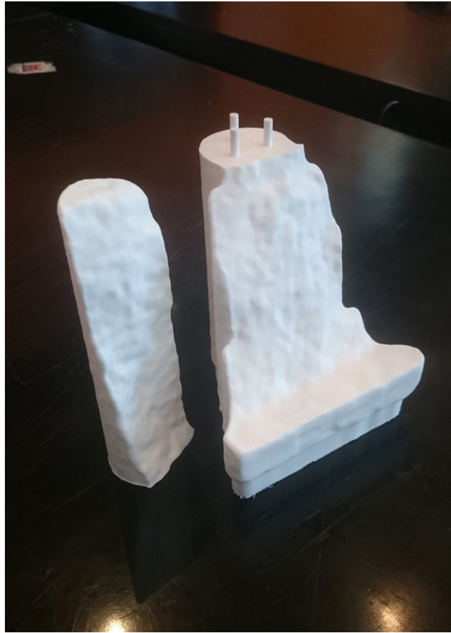
The two printed fragment parts did not need an adhesive to be joined together and would fit together readily.
