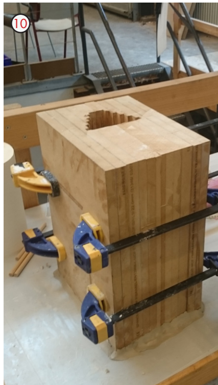
10. The pattern was placed approximately in the middle of the mold reinforcement and the setup was clamped shut using four bar clamps.
