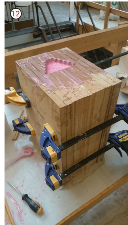
12. The newly poured silicone was then left to cure inside the mold reinforcement for 24 hours.
