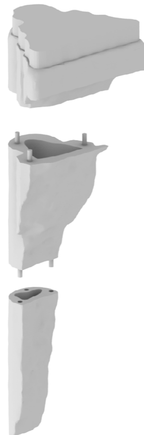
Figure 134. Three part model with cavity for Form 1+ Printer. Source: Author
