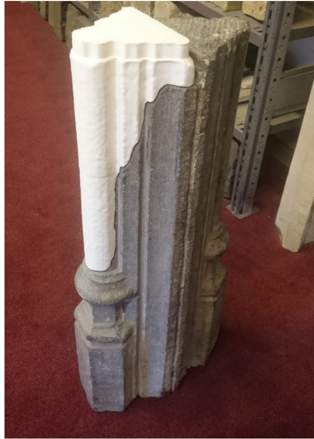
Interestingly, because the manufactured fragment fit the stone column so accurately, it did not require any adhesion or force to be kept in place.
