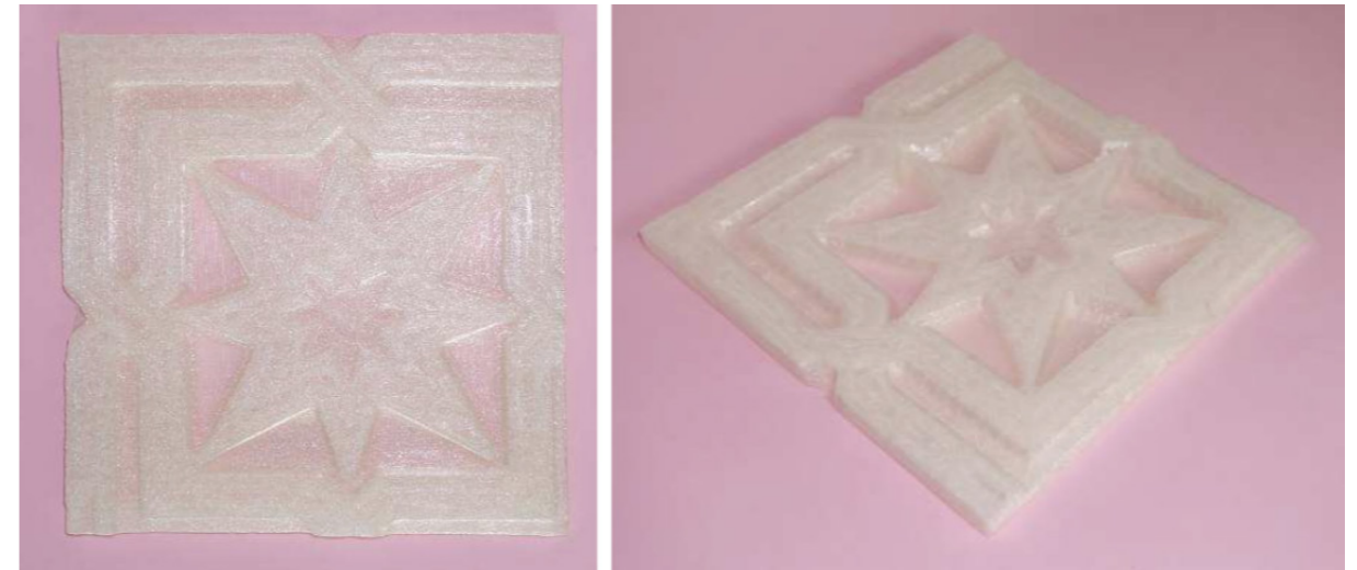
Figure 23. FDM Printing Result (PLA). Source: Adrian Gheorghiu
