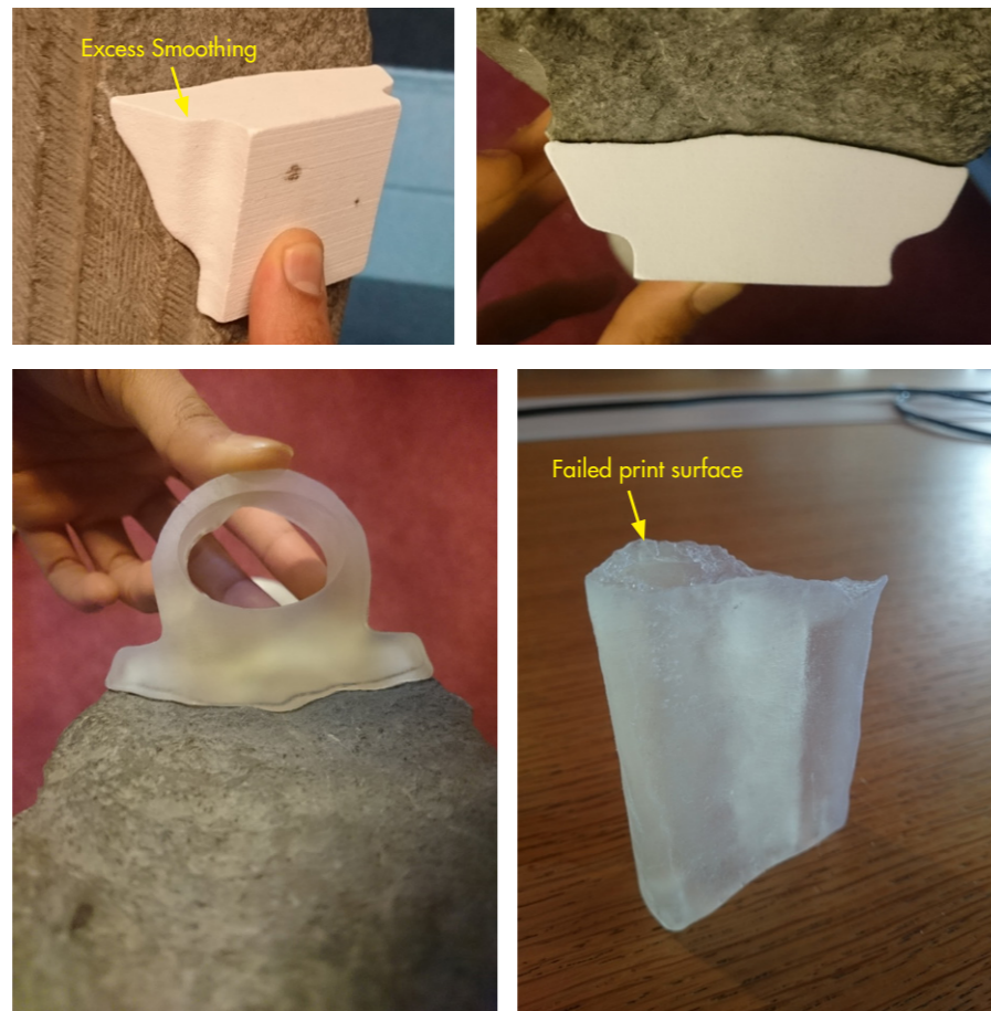
Figure 133. Testing Morphologies and Failed Prints. Source: Author
