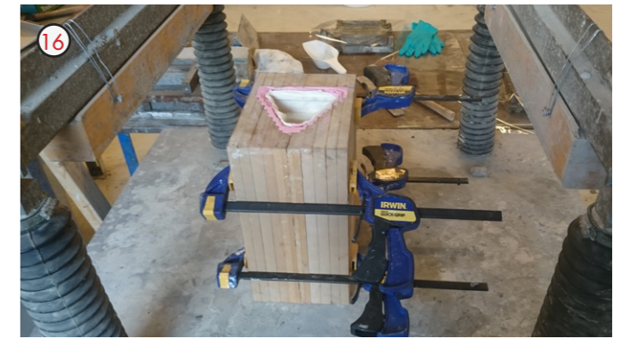
16. The mold setup was placed on a vibrating table to prepare for the casting process. The vibrating table helped ensure that no bubbles were trapped inside mold. Bubbles can potentially cause loss of detail and larger bubbles can result in improper casting.
