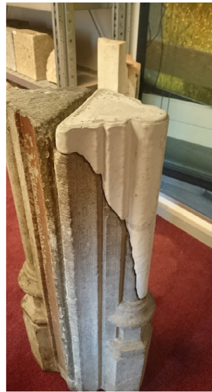
Fitting of the second cast, the lightening caused by the doubling of the pigment amount is visible.
