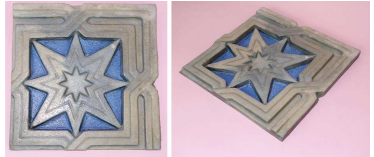
Figure 21. Pro-jet Printing Result. Source: Adrian Gheorghiu
