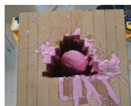
11. The silicone (with Mold Max 30 Part B) was slowly poured around the pattern to ensure that there are no gaps left behind. Care was also taken to ensure that the pattern did not move during pouring.
