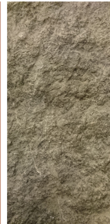
Figure 64. Close-up of fracture surface, the high frequency detail is visible. Source: Author
