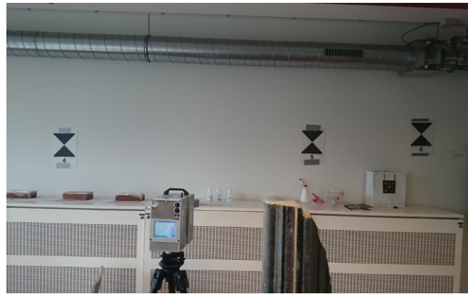
Figure 71. Printed Reference Markers. Source: Author
