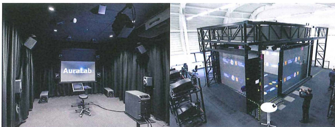
Figure 5 – Photographs of the upper hemisphere loudspeaker layout in Empa's AuraLab (left) and of the aixCAVE at RWTH Aachen University (right)
