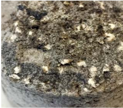
Figure 16. The surface of the FMFT column showing bitumen and salt crystals
