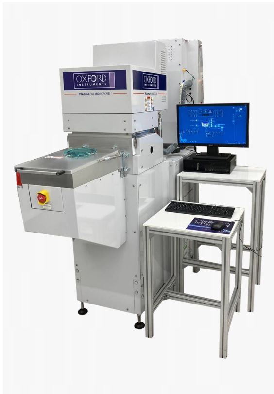
(a) The Oxford Plasma Pro 100. The side observation pane is visible on the right side of the ICP-PECVD. The optical fiber connected to the spectrometer looks through this pane.
