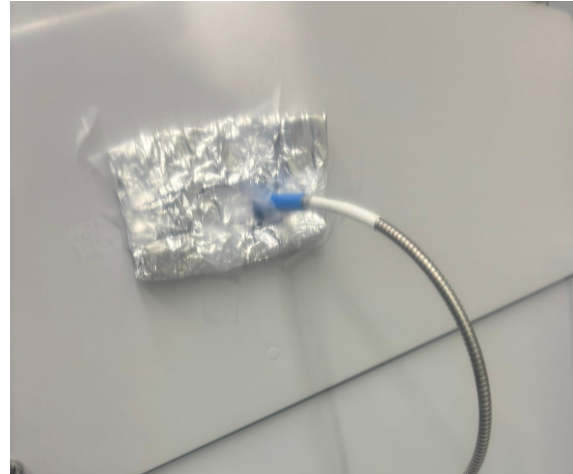
(b) The side observation pane through which an optical fiber connected to the spectrometer looks at the plasma during deposition. It is pierced through an aluminium sheet to remove any background light.
