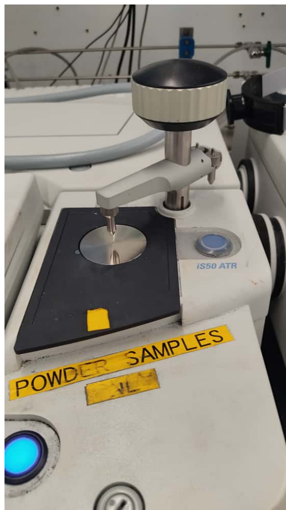
(b) Diamond crystal and pressure tip
