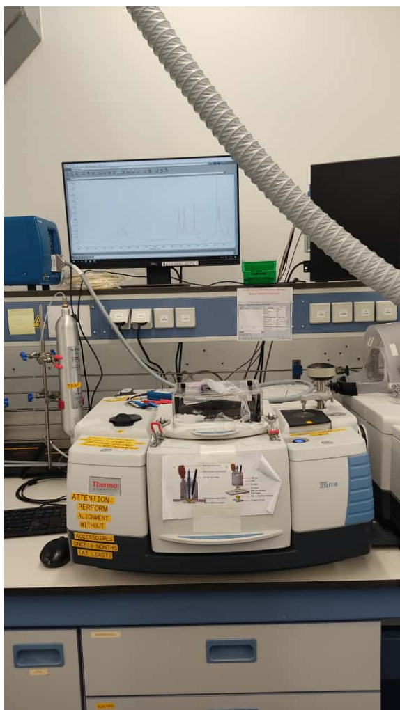
(a) Overall Setup-Nicolet iS50 FTIR Spectrometer
