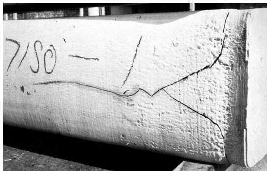
Fig. 19. Cold crack in a 7xxx DC ingot.
