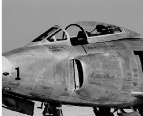
Figure 2.7: A scoop inlet mounted on the NACA research aircraft YF-93A [30].
