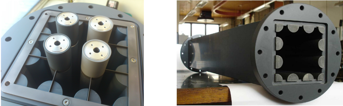
Figure 5.4: A section from the rod-bundle set-up, with a close-up of the rods, from Van Campen [6].
