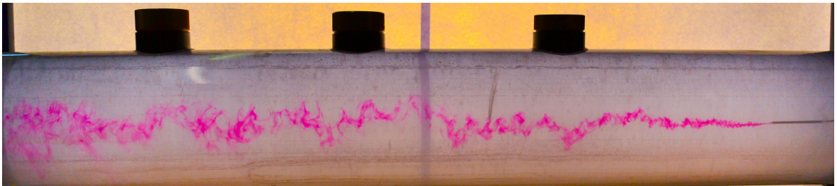
Figure 4.3: The tracer needs some development length, before it starts to follow the velocity field at the small scales. The flow goes from right to left.
