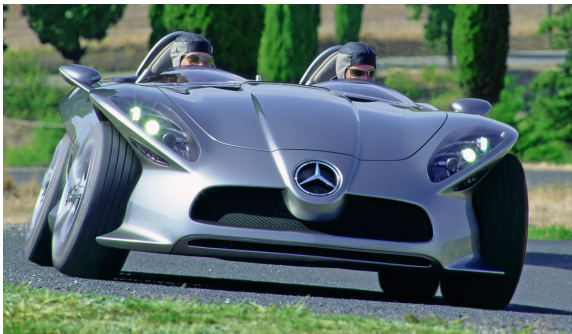
Figure 2.19: Mercedes F400 concept vehicle with active camber control [10].
