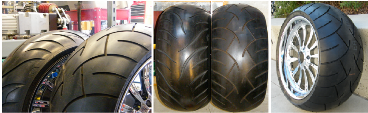
Figure 2.17: Hybrid motorcycle/car tire [11]. These tires might be a suitable option for an active camber mechanism. The smooth curve maintain the same contact area for a wide range of camber angles.
