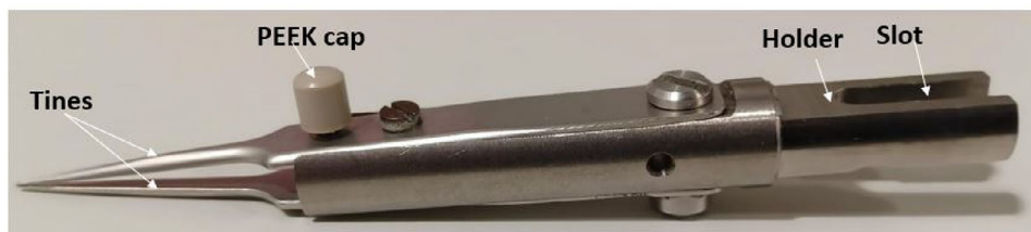
Figure 13. Photograph of the modified tweezer used in the setup.
