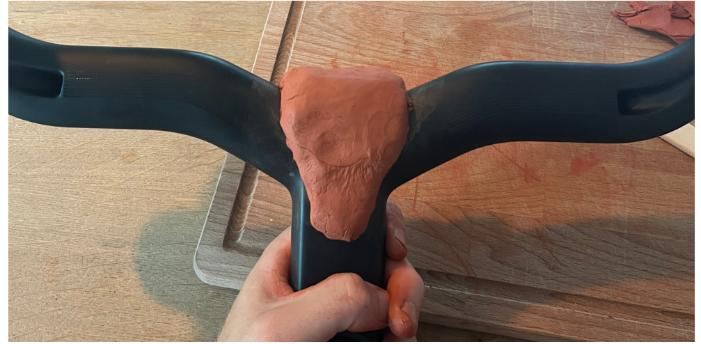
Figure 16: Clay model to copy handlebar curvature and transition
