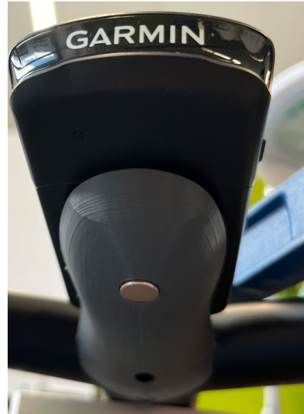
Figure 38: The magnet embedded in the BCM.
