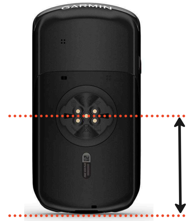
Figure 5: Distance between edge of computer and mounting centre, a parameter used to design the BCM.
