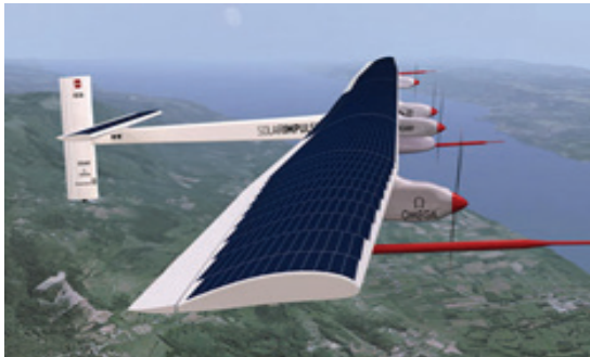
FIGURE A.13: LEFT IMAGE: SOLAR IMPULSE PLANE IS A PV-POWERED, SINGLE-PILOT AIRCRAFT (2009-2014). ITS WINGS ARE COVERED WITH 11,000 SOLAR CELLS, WITH A WINGSPAN OF 210 FEET. SOURCE: THE TECH JOURNAL, 2015. RIGHT IMAGE: HELIOS IS THE NASA'S PV-POWERED PROTOTYPE AIRCRAFT (1999-2003). IT WAS DESIGNED TO OPERATE AT EXTREMELY HIGH ALTITUDES USING BATTERIES AND HIGH-EFFICIENCY SOLAR CELLS SPREAD ACROSS THE UPPER SURFACE OF ITS 247-FOOT WINGSPAN. SOURCE: THE TECH JOURNAL, 2015.
