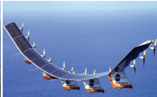
FIGURE A.13: LEFT IMAGE: SOLAR IMPULSE PLANE IS A PV-POWERED, SINGLE-PILOT AIRCRAFT (2009-2014). ITS WINGS ARE COVERED WITH 11,000 SOLAR CELLS, WITH A WINGSPAN OF 210 FEET. SOURCE: THE TECH JOURNAL, 2015. RIGHT IMAGE: HELIOS IS THE NASA'S PV-POWERED PROTOTYPE AIRCRAFT (1999-2003). IT WAS DESIGNED TO OPERATE AT EXTREMELY HIGH ALTITUDES USING BATTERIES AND HIGH-EFFICIENCY SOLAR CELLS SPREAD ACROSS THE UPPER SURFACE OF ITS 247-FOOT WINGSPAN. SOURCE: THE TECH JOURNAL, 2015.
