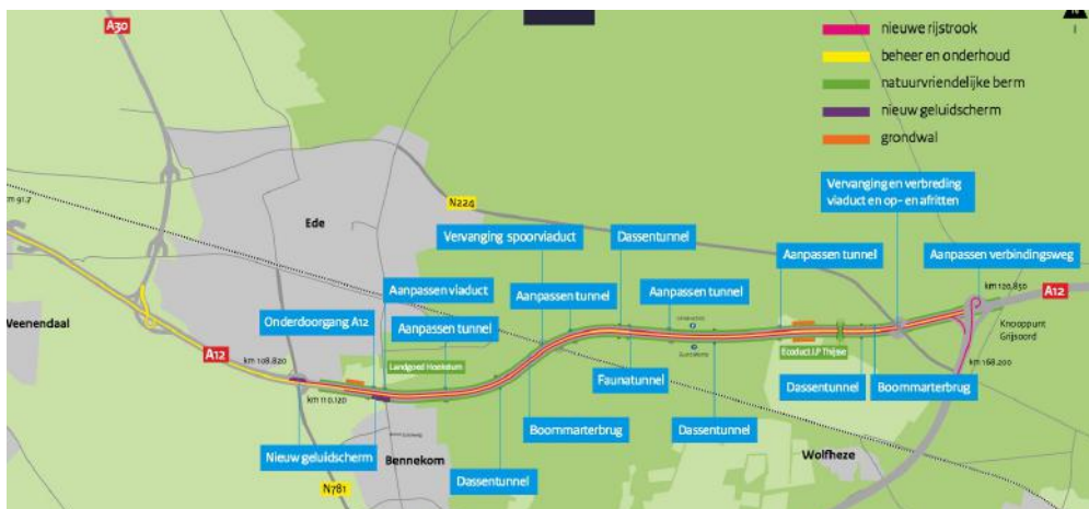
Figure 4.3. Track of project A12 Ede-Grijsoord (Heijmans, 2016)
