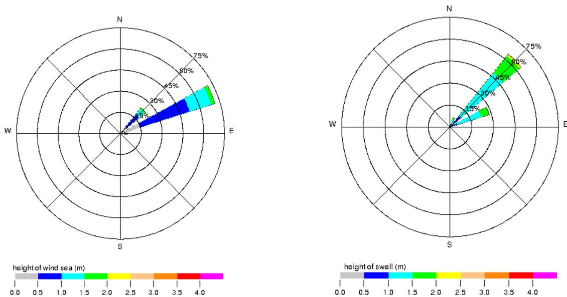
Figure B.3 Direction and wave height in April and May (Source: BMT ARGOSS, 2017).
