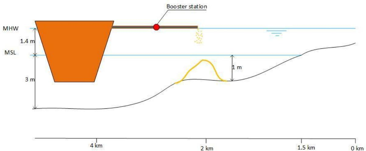
Figure 6.23 Construction method, placing of the chenier (Source: own illustration)
