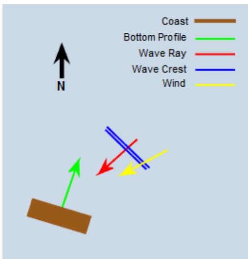
Figure B.10 Orientation of the bottom profile, wave- and wind direction with respect to the coast (Source: own illustration)
