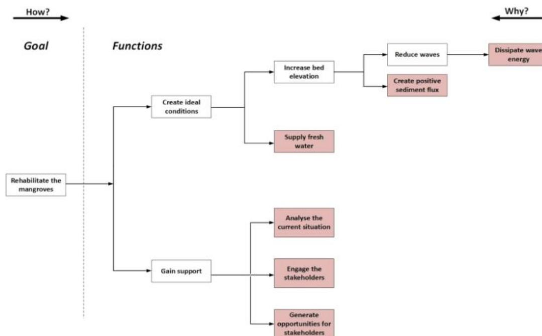
Figure 1.5 Functional analysis diagram (Source: own illustration)
