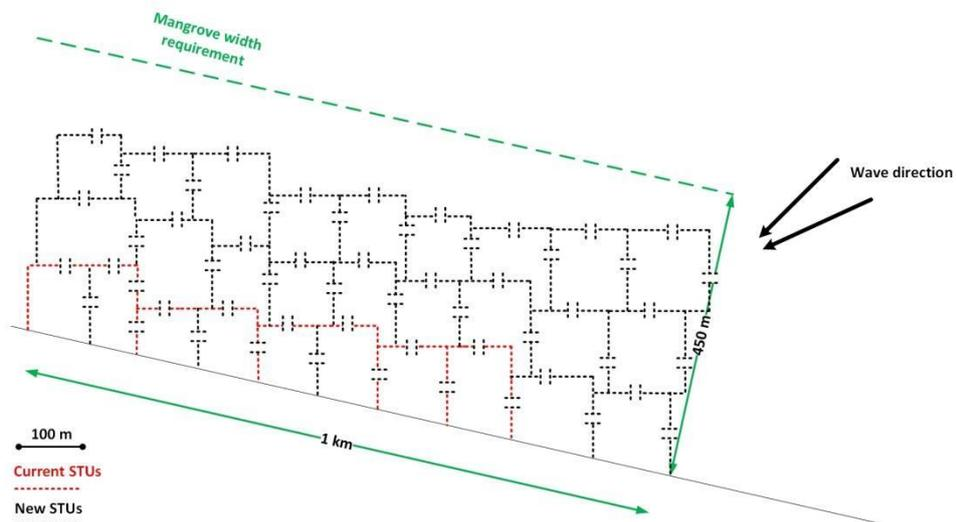
Figure 6.7 Phase 2 of construction STUs after required sedimentation in phase 1 is reached (Source: own illustration)
