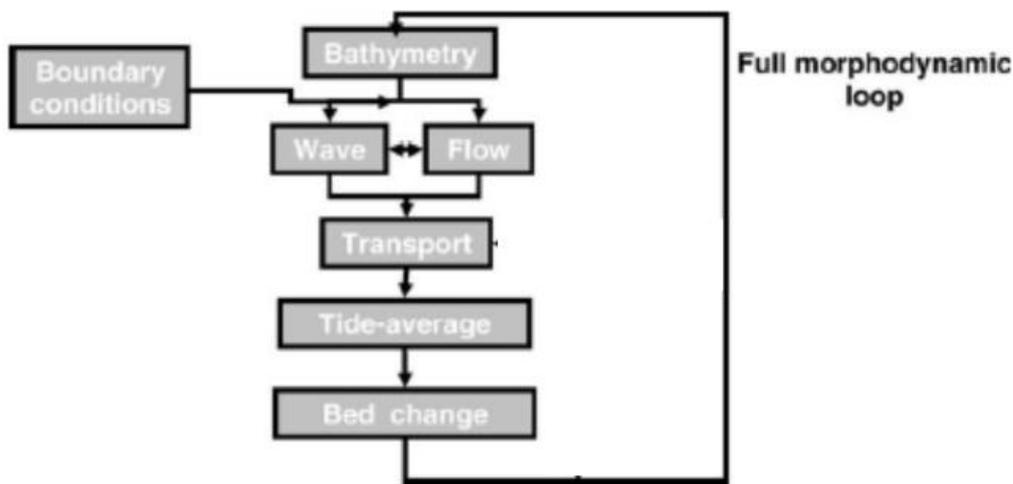
Figure 6.25 Morphodynamic loop in the Delft3D model, (Source: Walstra, 2017)
