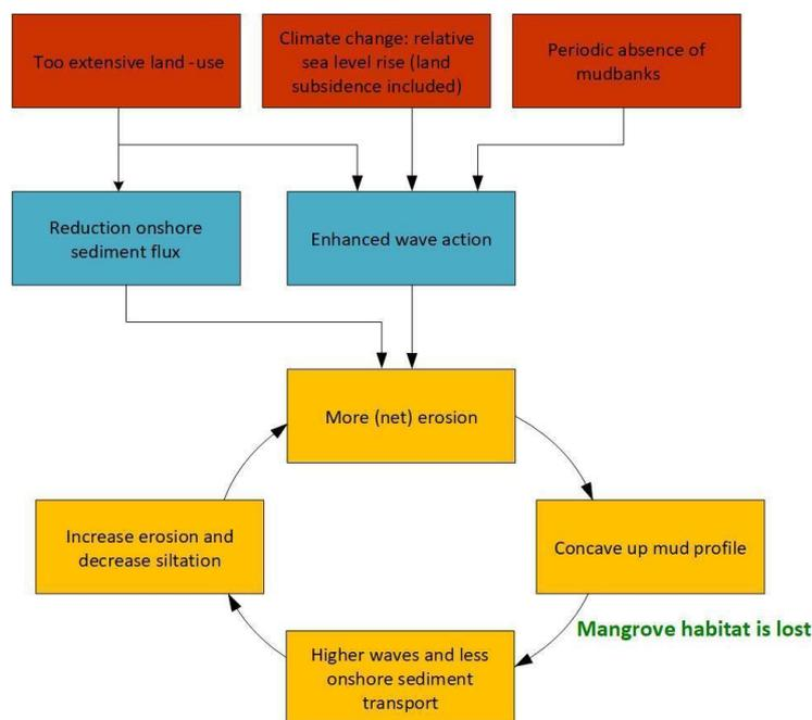
Figure 1.2 Main causes of erosion in Suriname (Source: own illustration)
