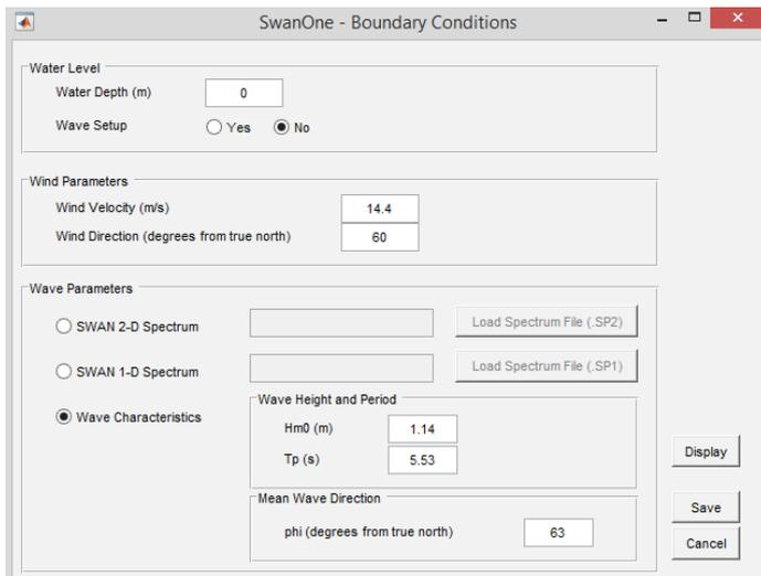
Figure B.9 Input parameters in SwanOne (Source: own illustration)
