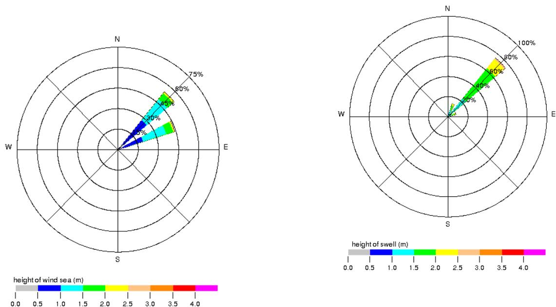
Figure B.2 Direction and height of swell and wind waves during Winter (January-March) (Source: BMT ARGOSS, 2017).
