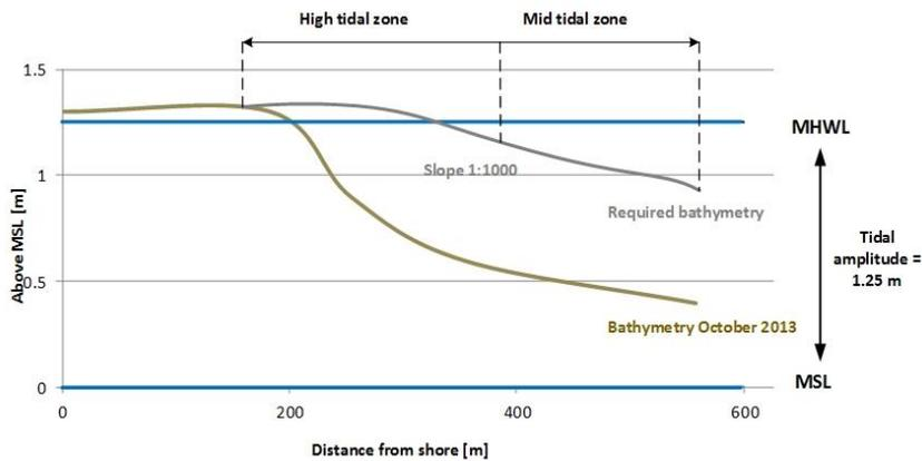
Figure 4.14 Current bathymetry and required bed level (Source: own illustration)
