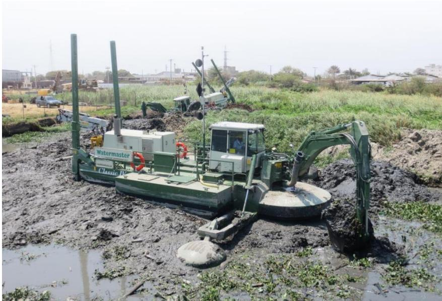
Figure 6.20 The watermaster on soft soil (Source: Watermaster, n.d.)
