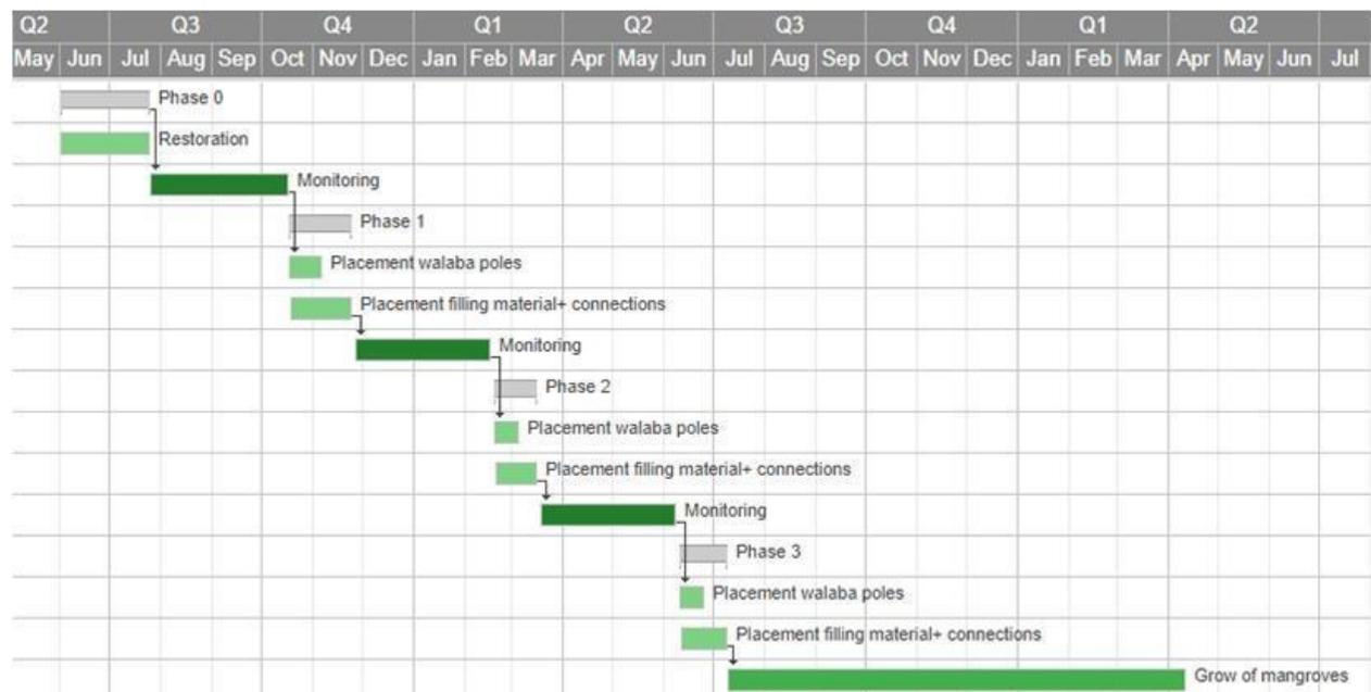
Figure 6.13 Gantt Chart of the construction for Preliminary design 1 (Source: own illustration)
