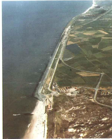
The tip of North Holland has been receding for centuries. The protruding Hondsbosche sea dyke offers evidence of this fact.
