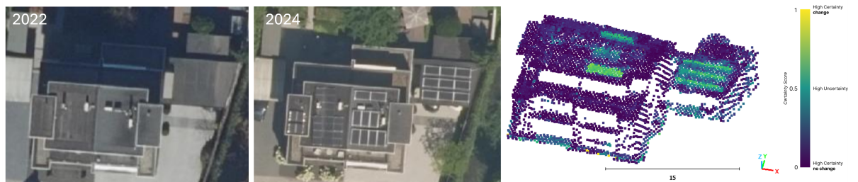
Figure D.15.: Detection of angled solar panels installed between Rotterdam 2023 and AHN5 . Panels placed at an angle are detected with moderate to high certainty of change. Those aligned with the roof slope are less reliably detected. Orthophotos from 2022 and 2024 are shown for reference point cloud dataset . Source: Beeldmateriaal Nederland .
