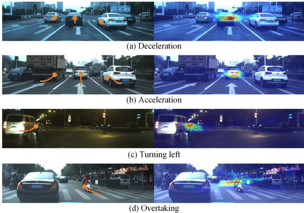
Fig. 8. The recognition effect of the proposed framework of four scenarios.
