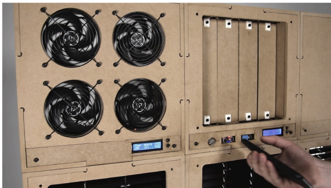
Figure 12. (Video3) The ventilation flaps close due to noise pollution and mechanical ventilation is activated.
