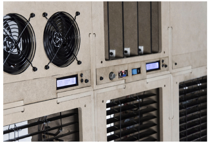
Fig. 2. The front of the prototype with visible sensors, LCD displays and LEDs.
