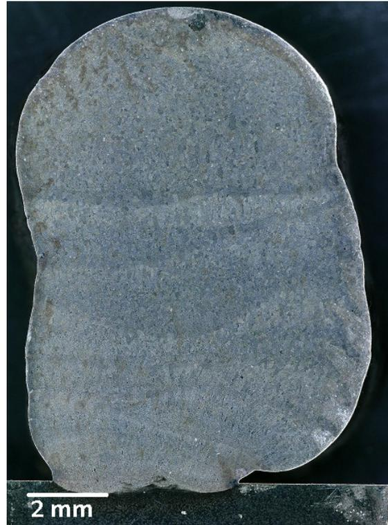
**Figure 25:** Macrostructure of cross-section of 6-layer deposits on NAB base plate. Characteristic WAAM based layer microstructure bands are observed.
