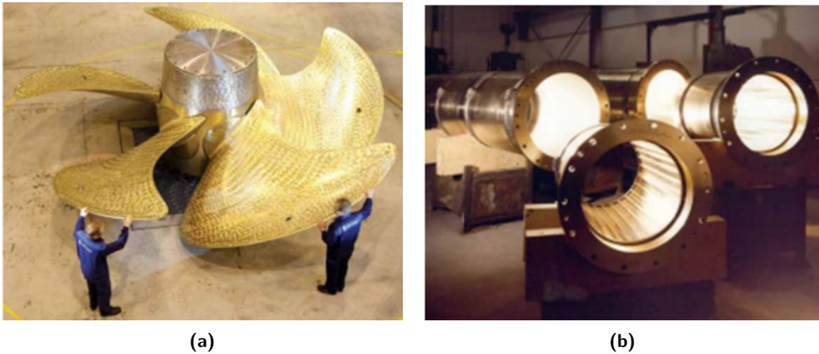
**Figure 2:** Applications of aluminium bronzes (a) ship propeller (b) offshore pipeline [12]
