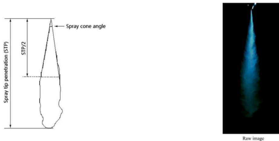
Figure A.3: Spray tip penetration (STP) and spray cone angle definition used by [83], p.10
