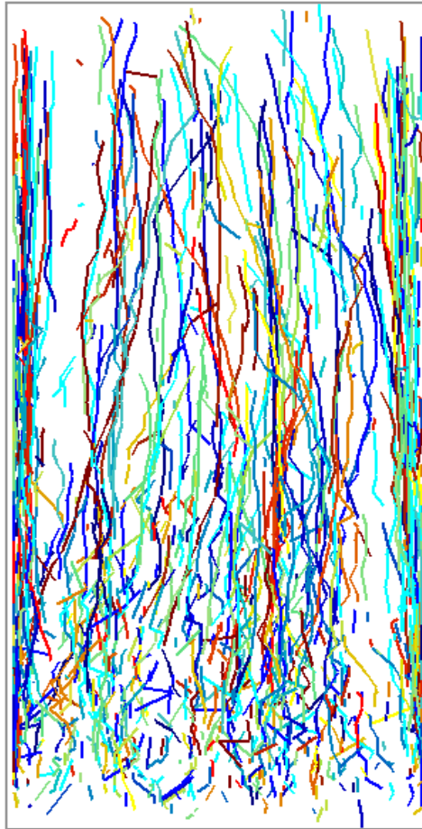
The chaotic tracks of bubbles rising through a fluidized bed, when no electric field is applied. The image was generated from the simulations presented in this chapter.
