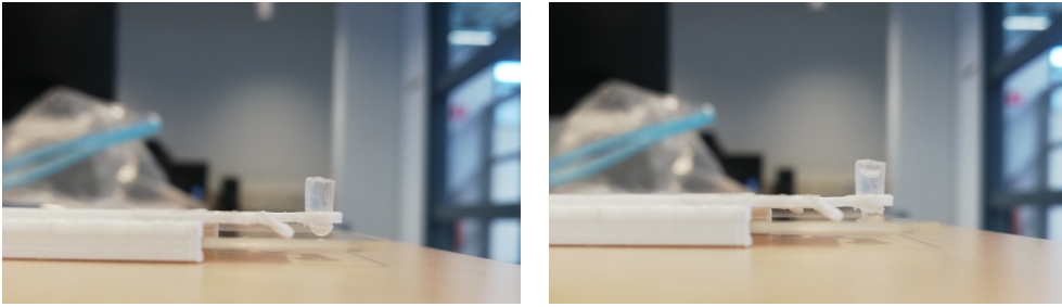
Figure 89: The drop tends to flow 'fall out' of the tube, resulting in dropping more blood than desired.
