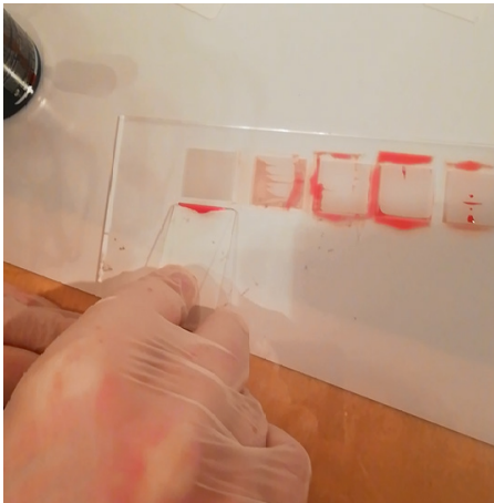
Figure 64: Use of the Notch. A blood drop is placed in front of the notch, after which it is spread.
