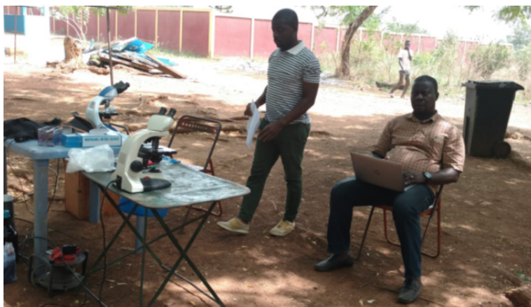
Figure 17: A lab set-up under the trees increases the risk of environmental contamination.
