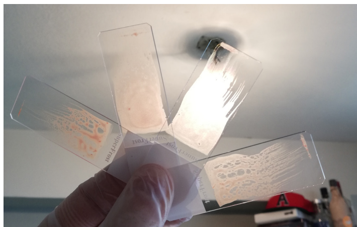
Figure 67: Unclean slides lead to poor quality smears.
