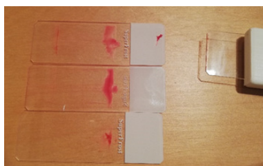
Figure 57: Use of the Mimicker. The slide is pushed through the device, spreading the blood.
