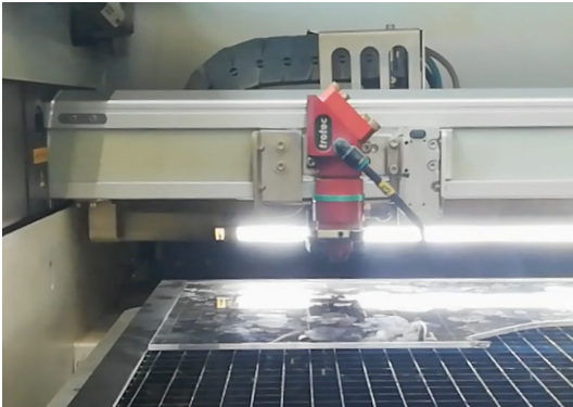
Figure 62: A laser cutting, 'engraving' the notches in the plexiglass sheet.
