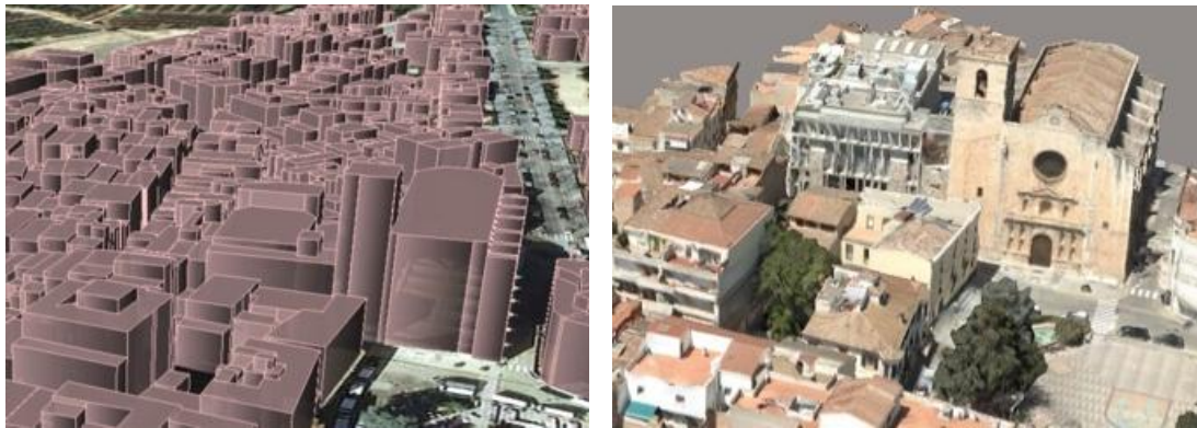
Figure 4 – Current LoD1 model without textures and the LoD2 model texturized using oblique images
