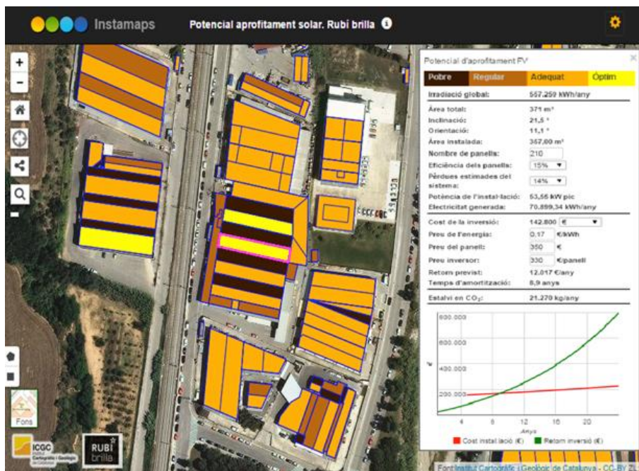
Figure 6 – Application to provide the solar potential of buildings based on LiDAR data
