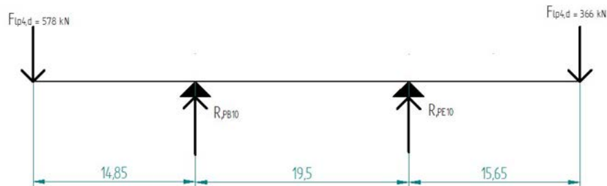
Figure C.12: Horizontal force balance, pinned connection
