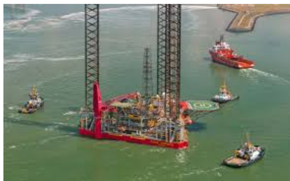
Figure 2.16: The Energy Endeavour towed to shore after topside removal [? ]
