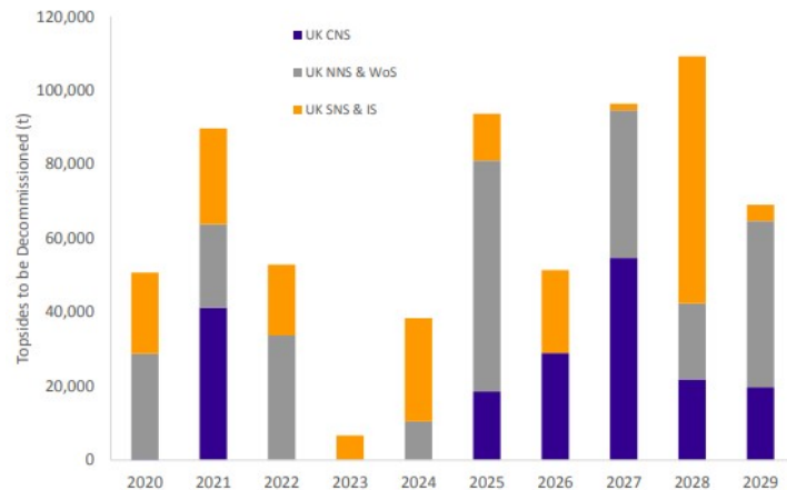
Figure 2.4: Topsides weight to be removed in the UKCS [29]
