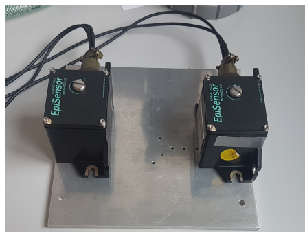
Figure 6.8: Measurement check to confirm equal input signals.
