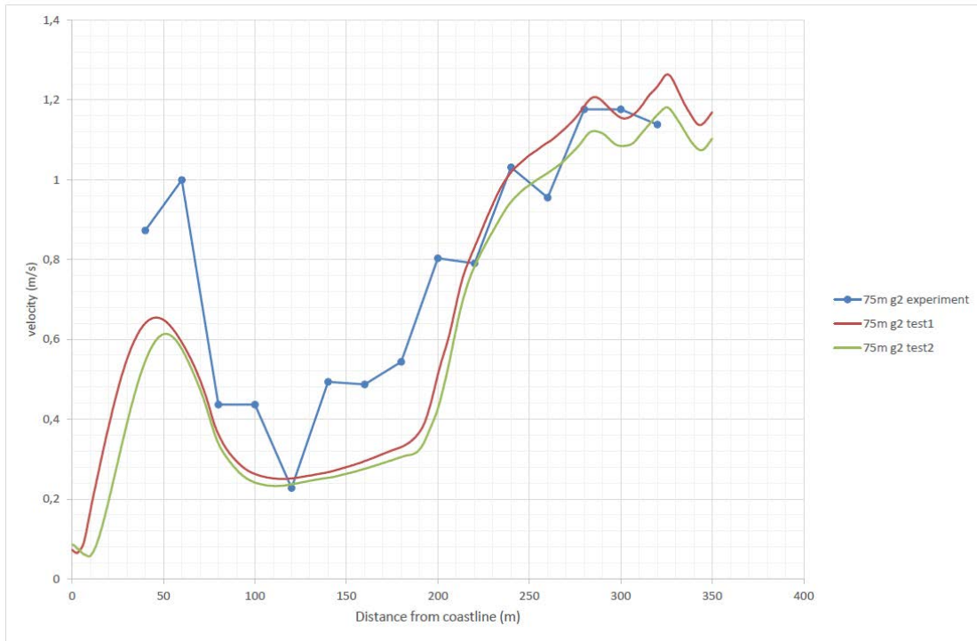
Figure B.10 Longshore current profile at a distance of 75 m from the pile groin 2
