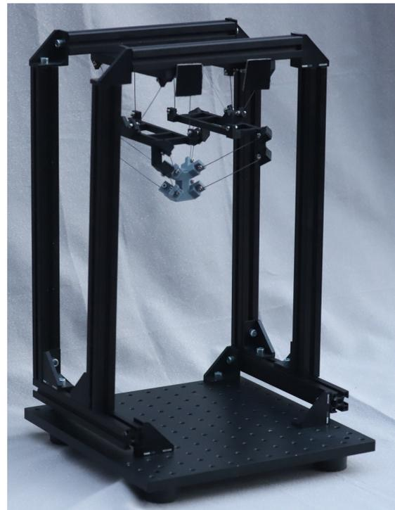
**Figure E-9:** Demonstrator frame set up (Frontview at an angle); Gray body is end-effector, two black bodies the IMBDs.
