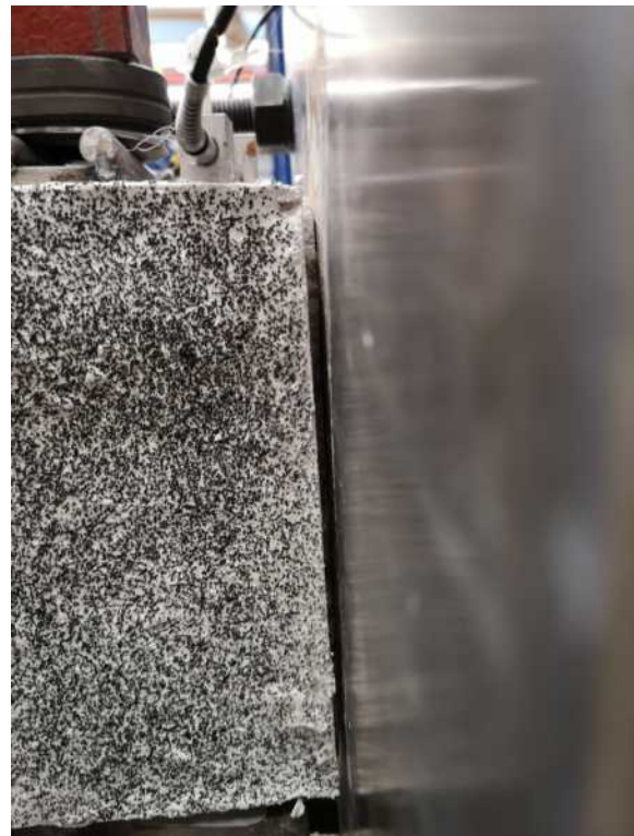
(b) Specimen inside the experimental setup clearly shows no contact between the steel plate and the overlay material.
