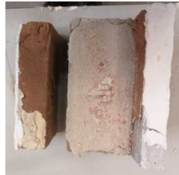
(b) Failed interfaces specimen A, 30 mm SHCC overlay.
