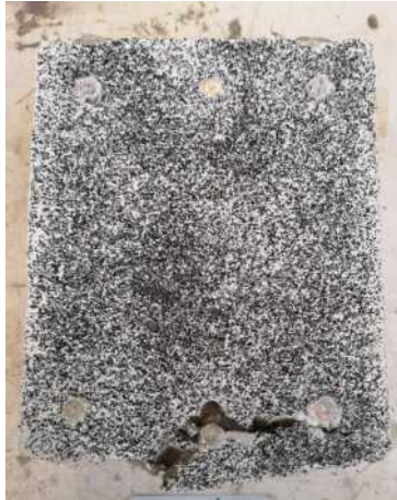
(a) Failure pattern 10 mm SHCC specimen with screws; specimen A.
