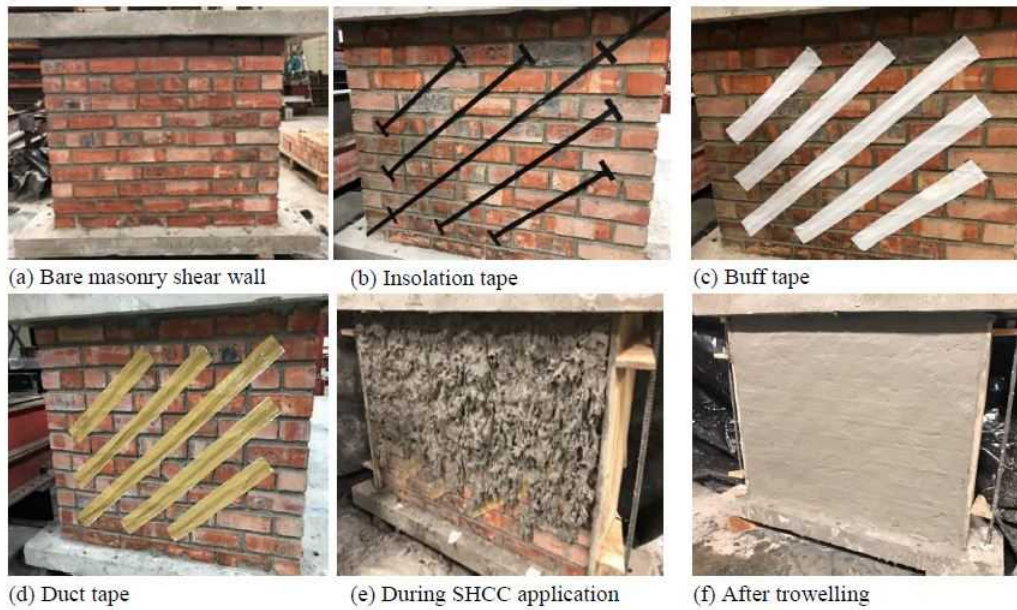
Figure 2.32: Manufacturing of masonry walls with debonded strips [39].
