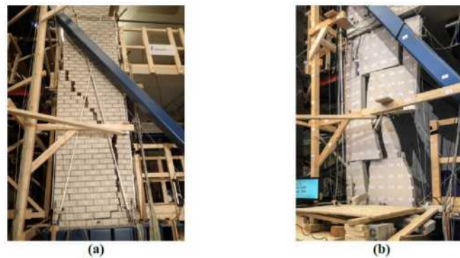
Figure 2.9: Main damage in wide piers at ground floor: (a) CS brick masonry assemblage; (b) CS element masonry assemblage [15].
