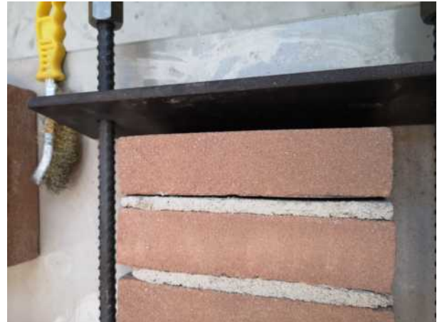
Figure 3.5: Delaminated masonry unit, masonry beam specimen
