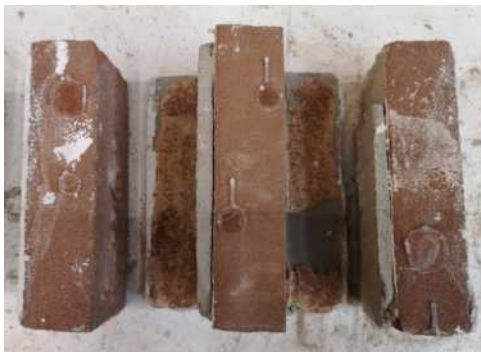
(a) Failed interfaces specimen A, 10 mm SHCC overlay.
