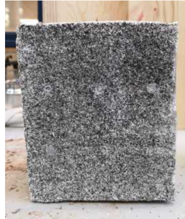
(b) Failure pattern 30 mm SHCC specimen with screws; specimen A.
