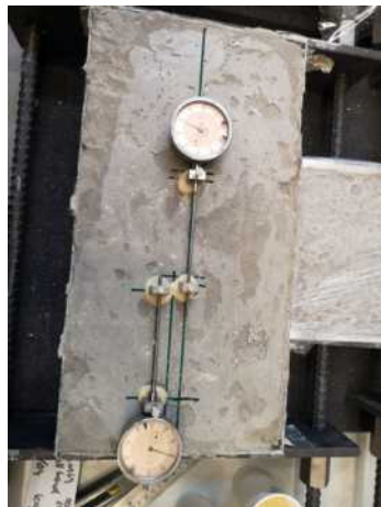
(a) Strain gauges restrained shrinkage masonry beams, laboratory conditions.
