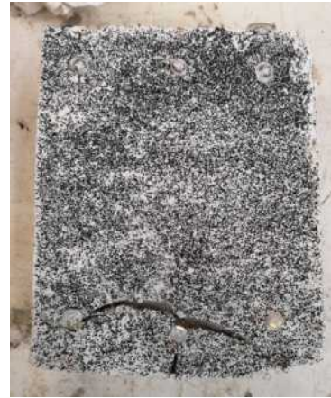
(b) Failure pattern 10 mm SHCC specimen with screws; specimen B.
