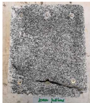
(d) Failure pattern 30 mm SHCC specimen with screws; specimen C.
