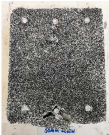
(c) Failure pattern 30 mm SHCC specimen with screws; specimen B.
