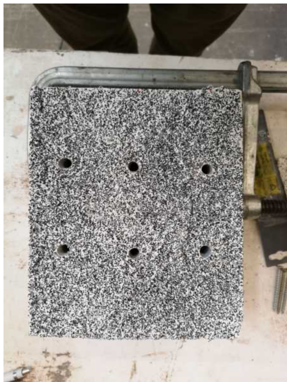
(a) Drilled holes for installation of screws, 70 mm edge distance.
