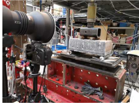
(b) Front view retrofitted masonry beam with the DIC pattern applied.
