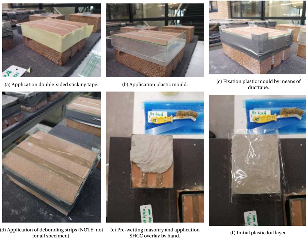
Figure 3.9: Overview general casting procedure SHCC overlay.
