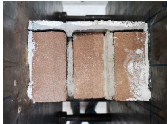
(b) Top view specimen after testing.
