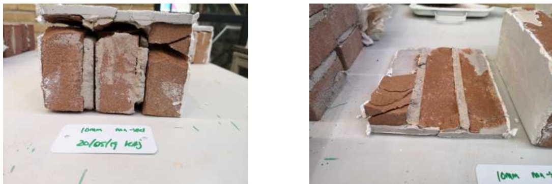
Figure 6.10: Overview failed specimen only SHCC-masonry interface glued. Overlay thickness = 10 mm, specimen B. Pre-compression = 1.0 Mpa.
