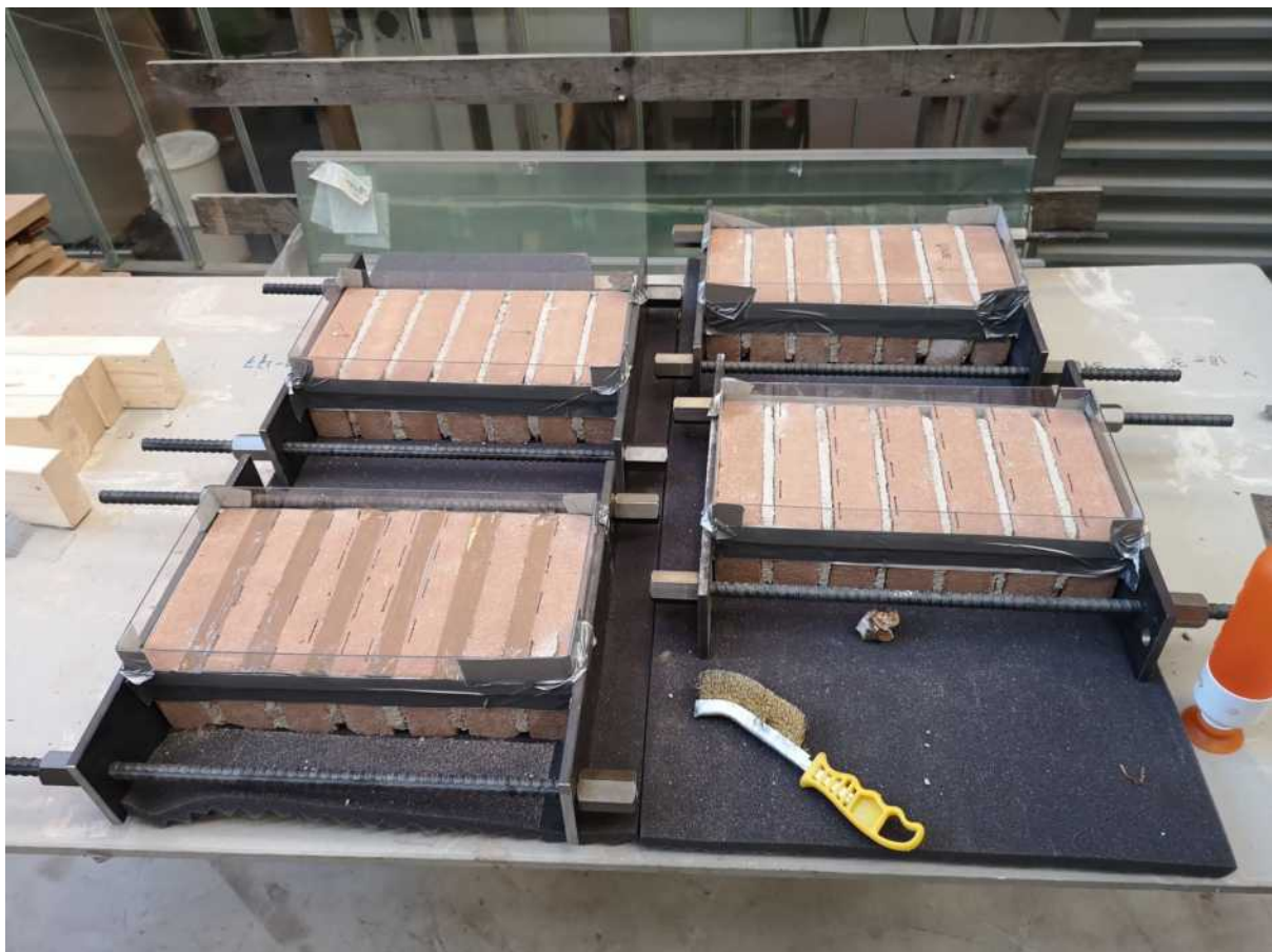
Figure 3.6: Final configuration masonry beams before casting SHCC overlay.
