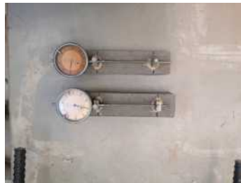
(b) Strain gauges free shrinkage SHCC prisms, laboratory conditions.
