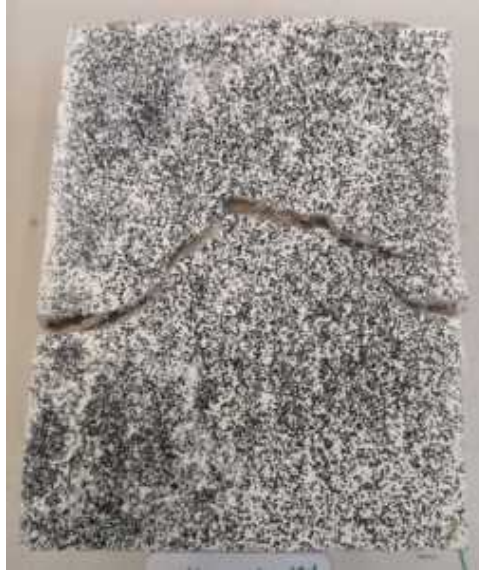
(c) Picture specimen after re-testing with glued interfaces.
