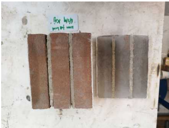
(c) Front view specimen after testing, delaminated SHCC overlay on the left.
