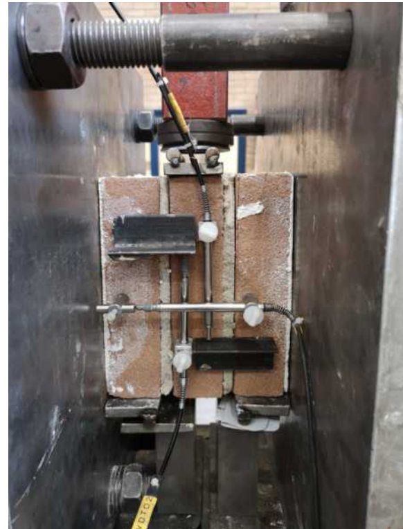
(b) Picture LVDT locations masonry triplet specimen.
