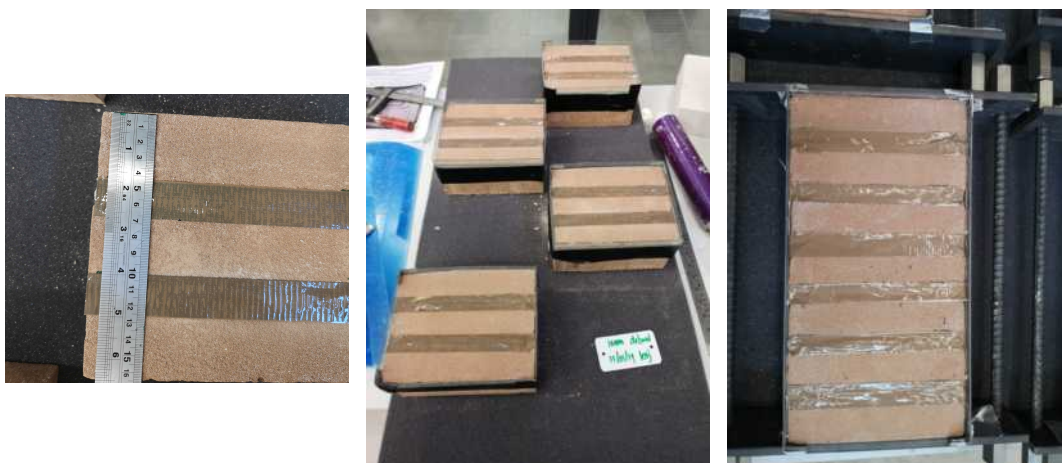
Figure 3.7: Applied tape on top of the mortar joints for several specimen (both masonry triplets and beams).
