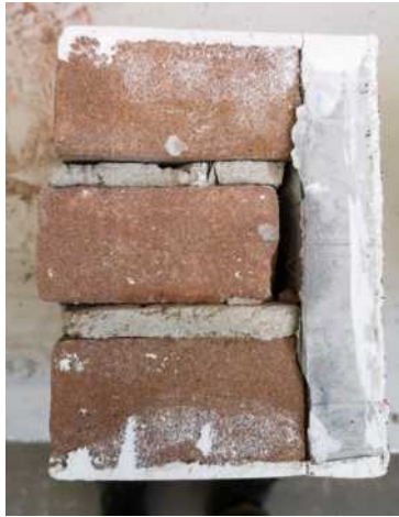
(a) Top view rotation of central unit; specimen A.
