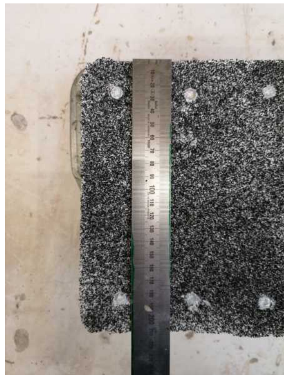
(b) Installed screws, 30 mm SHCC overlay, 25 mm edge distance.
