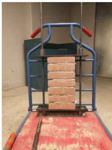
(a) Masonry beam in steel supporting frame.
