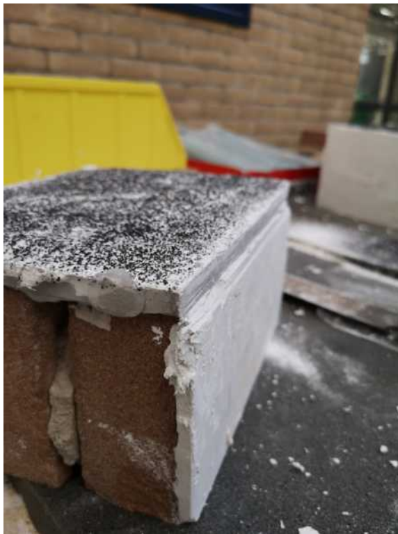
(a) Gypsum layer only applied to masonry material.
