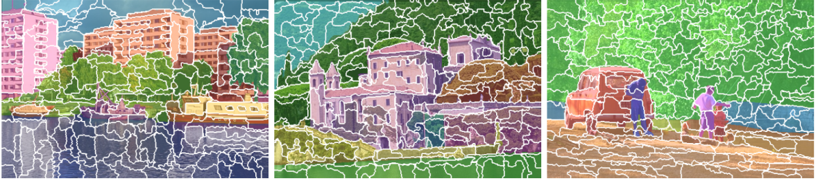
Figure 3-3: SEEDS over-segmentation results showing high quality superpixels. From (Van den Bergh et al., 2015)
