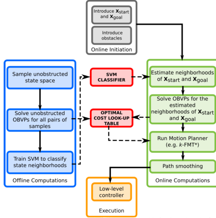
Figure 2-1: The real-time framework for kinodynamic planning and control of the quadrotor, from Allen et. al. (R. Allen & Pavone, 2016)
