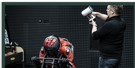
Measuring & 3D scanning rider
