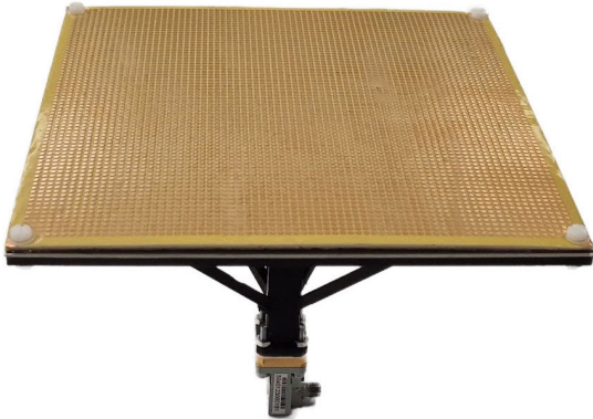
Fig. 16. Photograph of the assembled prototype showing the top layer of the four-layer ADL over a ground plane in a mount that holds the WR28 waveguide.
