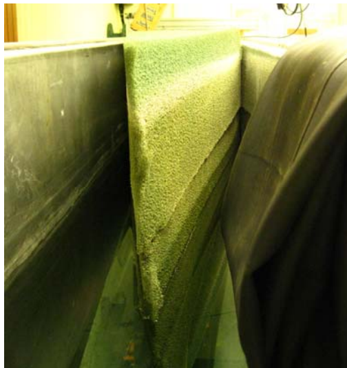
Figure 3-7 Absorption system used in the wave flume
