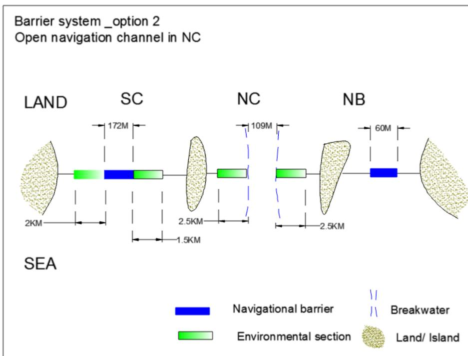
Figure K- 2. Barrier system option 2 – open navigation channel in North Channel
