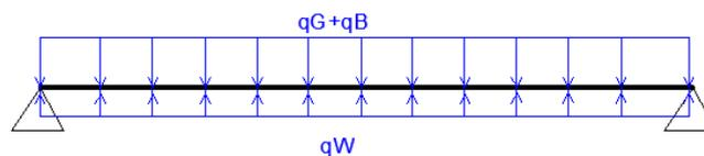
Figure 9- 26. Gate resting on vertical supports modeled as a beam
