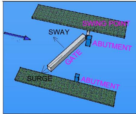
Figure 9- 31. Restricted motions of floating gate during closure
