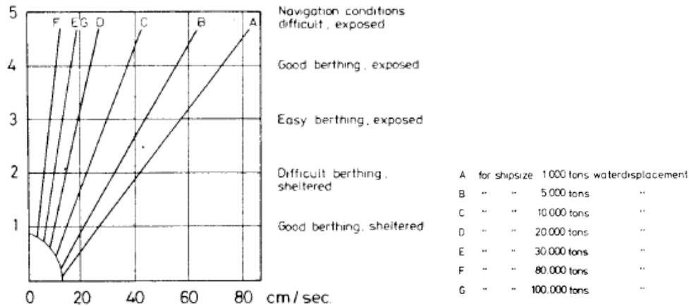
Figure 9- 38. Berthing gate velocity
