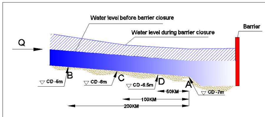
Figure 7- 9. Water Profile before and during barrier closure (not to scale)
