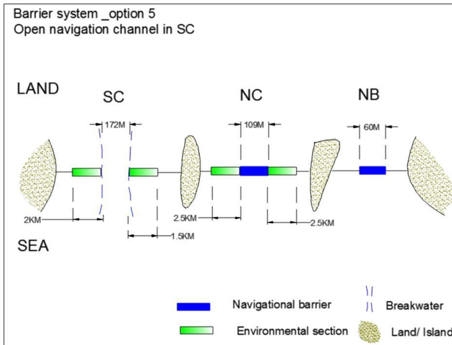
Figure K- 5. Barrier system option 5 – open navigation channel in South Channel
