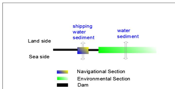
Figure 7- 2. Schematized barrier system in Yangtze Estuary as an entity
