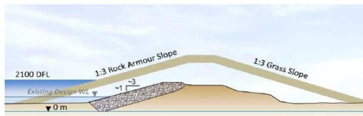
Figure 5- 4. Typical Cross Section of Sea Dike (Source: (Ministry of Environment of British Columbia, 2003))
