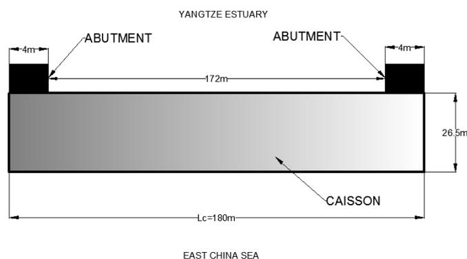
Figure 9- 22. Barge gate rested on the abutments during a storm
