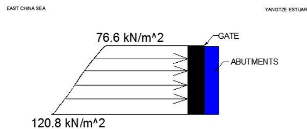
Figure 9- 24. Resultant distributed loads on the immersed gate when gate resting on abutments horizontally
