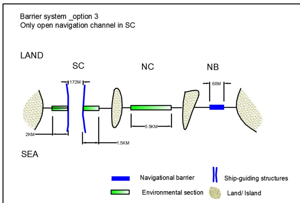
Figure 7- 12. Schematic plan view of open option
