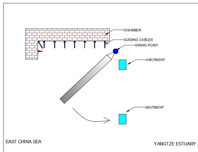
Figure 9- 4. Bird view of floating gate during closing process, not to scale
