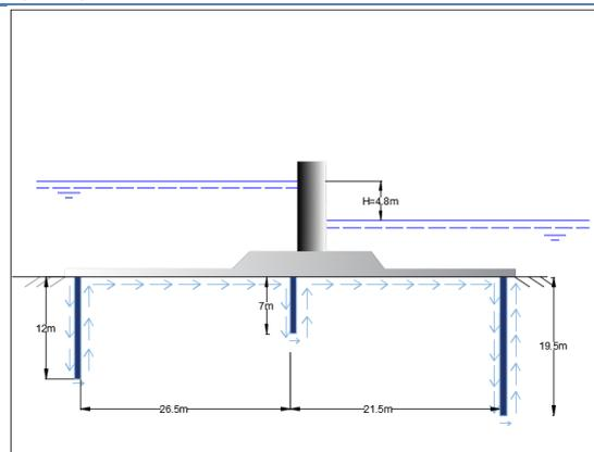
Figure 9- 42. Cross section of barrier and seepage screens
