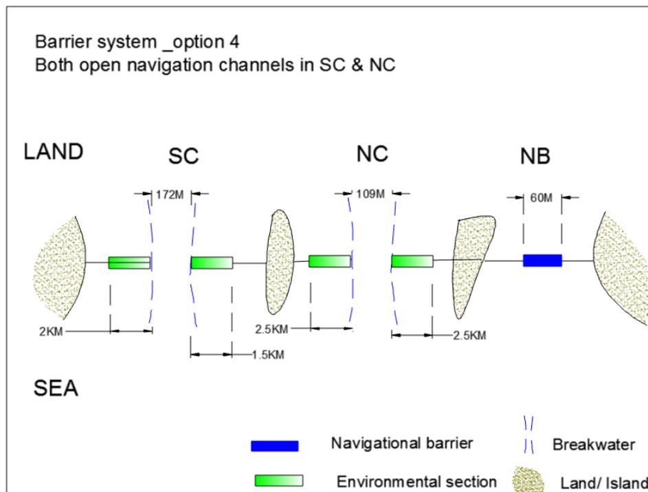
Figure K- 4. Barrier system option 4 – both open navigation channels in South Channel and North Channel
