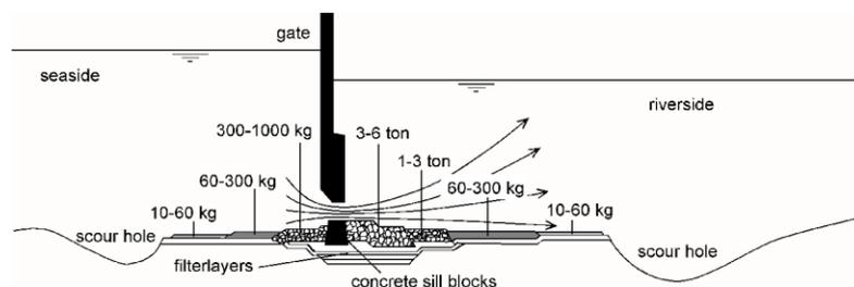
Figure 10- 5. Cross section bed protection of Maeslant barrier (Schiereck, 2001)
