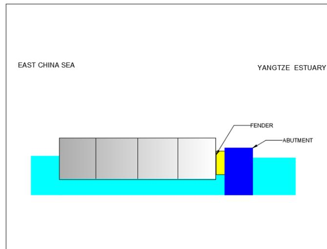
Figure 9- 3. Side view of floating gate during closing process, not to scale
