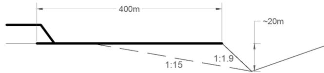
**Figure 10- 15. Scour hole behind bed protection**
