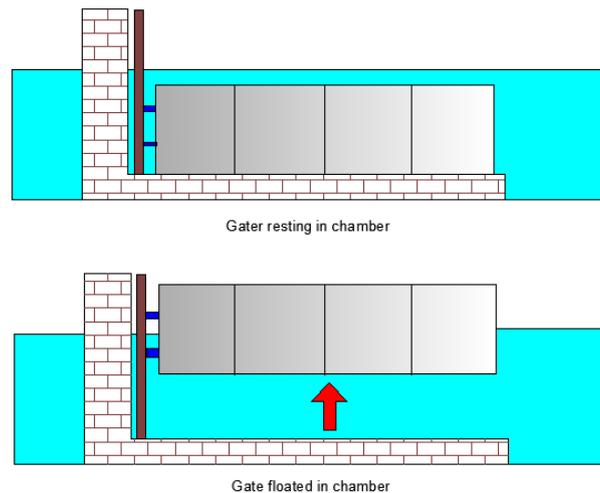
Figure 9- 5. Barge gate in open position, not to scale (cross section 1-1')
