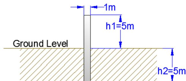
Figure E- 3. Typical Floodwall Cross Section Applied to Shanghai
