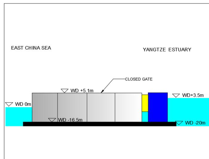
Figure 9- 9. Closed gate after storm condition, not to scale (cross section 3-3')
