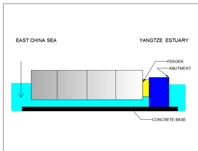
Figure 9- 6. Gate during immersion, not to scale (cross section 3-3')
