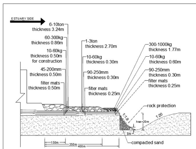
Figure 10- 11. Designed bottom protection in the estuary side behind opening of open option
