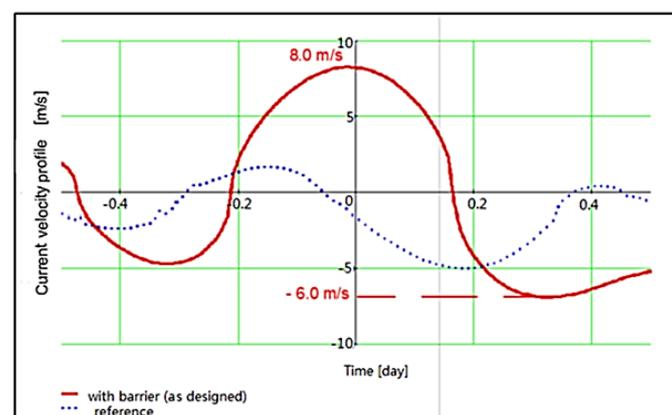
Figure 7- 14. Current velocity in the channel in open navigation channel option in design storm conditions (navigation channel width 375m)
