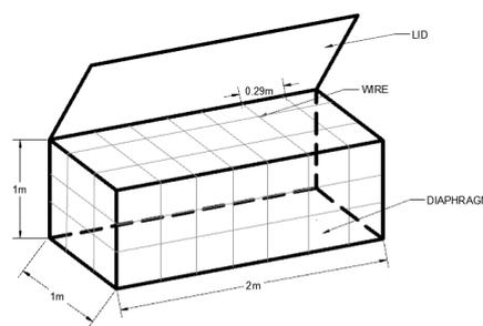
Figure 10- 9. Box gabion dimensions
