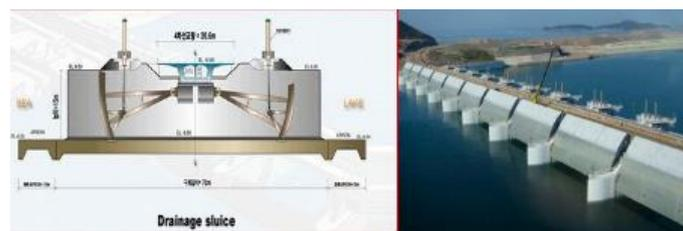
Figure 4- 7. Cross Section of Sinsi and Garyeok sluices
