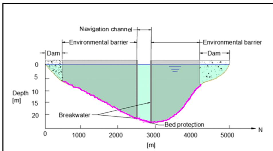
Figure 10- 2. Schematic front view of the 'open-option' in the South Channel (not to scale)
