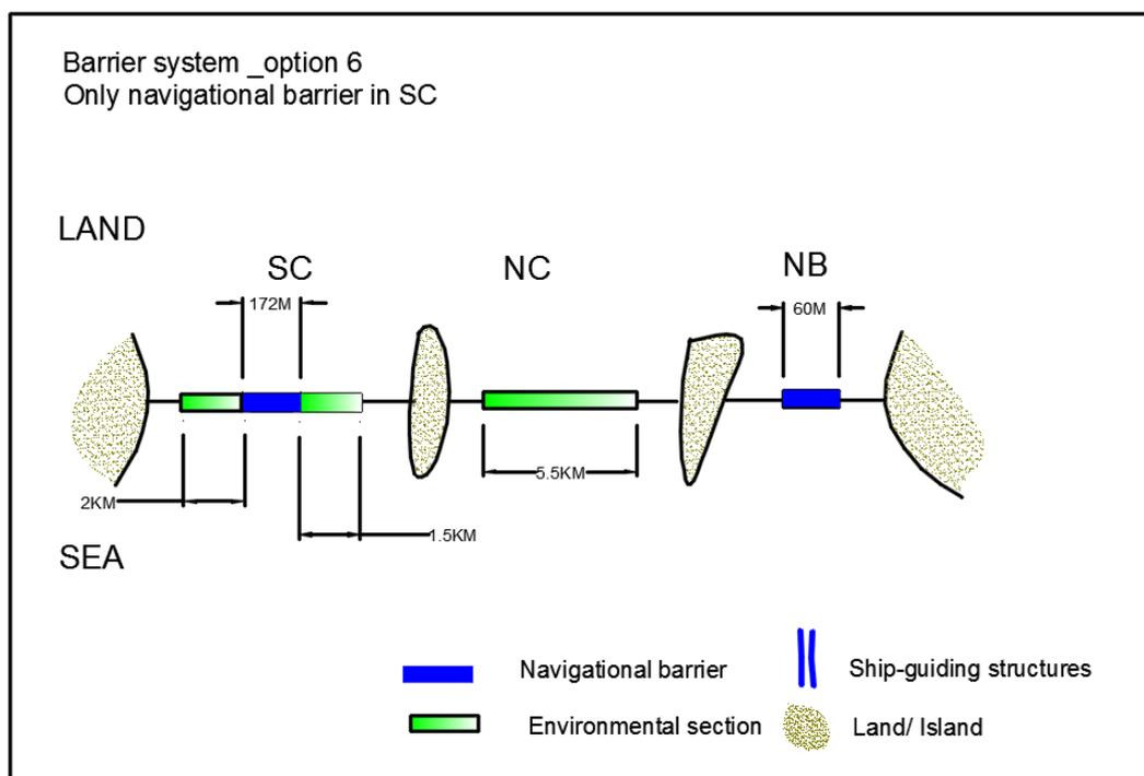
Figure 9- 1. Schematic plan view of gate option
