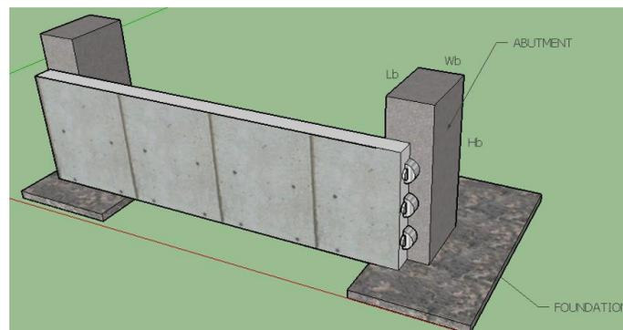
Figure 9- 36. Overview of gate resting on abutments (not to scale)
