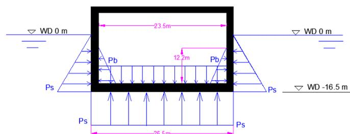
Figure 9- 19. Hydrostatic force scheme during immersion to WD-16.5 m at final location
