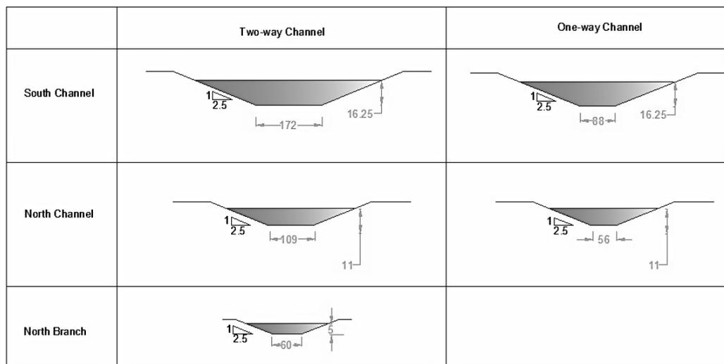
**Figure 7- 4. Proposed navigation channels cross sections**
