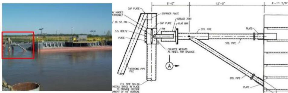
Figure 9- 33. Articulation system of the Bayou Lafourche swing gate (Labeur, 2007)
