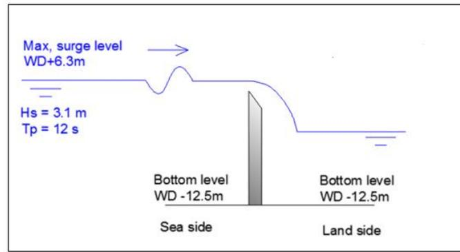
Figure 8- 3. Modeled lifting gate and designed conditions
