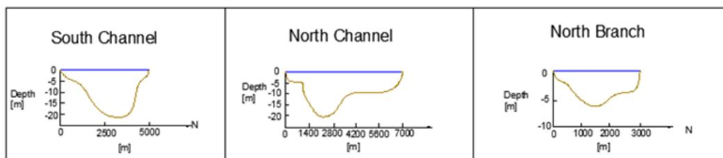
Figure 6- 1. Depth profiles of three channels in the Yangtze Estuary
