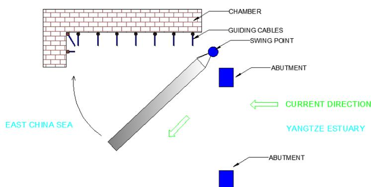
Figure 9- 10. Plan view of floating gate after storm condition, not to scale
