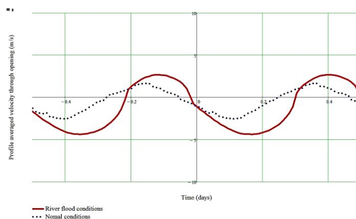
Figure 9- 40. Profile velocity through opening when all gates are opened (positive direction: from sea to the estuary)
