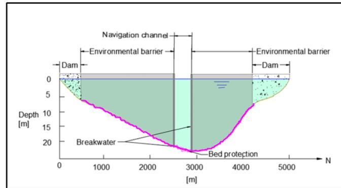
Figure 8- 2. Schematic front view of a barrier with open navigational section in the South Channel (not to scale)
