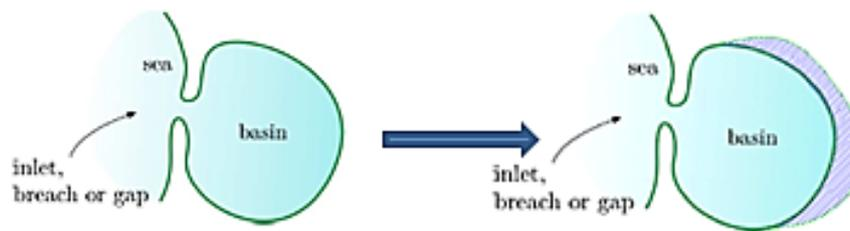
Figure 7- 7. Lift: original discrete system; Right: modified discrete system with additional storage area
