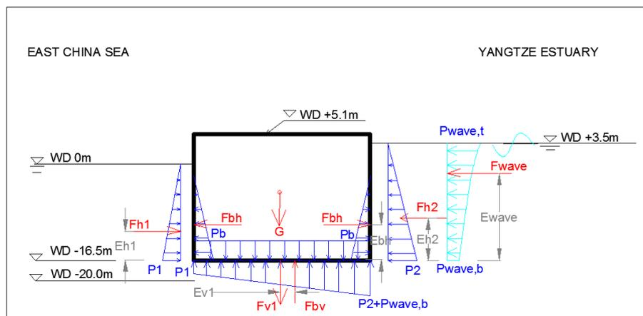
Figure 9- 27. Force scheme of immersed gate due to hydraulic forces (negative head)
