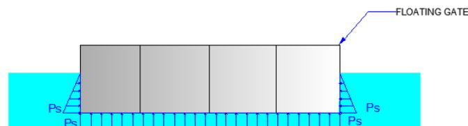
Figure 9- 17. Floating caisson during transport
