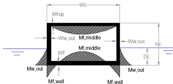
Figure 9- 15. Moment scheme on a floating caisson
