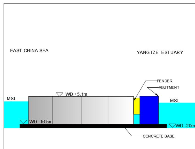
Figure 9- 7. Closed gate during normal conditions, not to scale (cross section 3-3')
