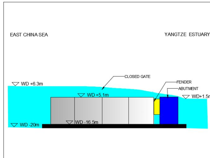
Figure 9- 8. Closed gate during storm conditions, not to scale (cross section 3-3')
