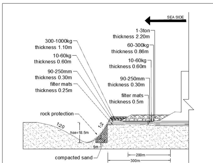
Figure 9- 41. Section view of designed bottom protection at both sides over the whole barrier length
