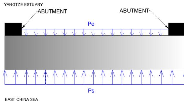
Figure 9- 23. Loads scheme on gate when rested on abutments
