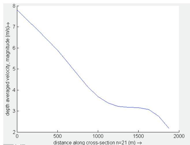
Figure 10- 4. Depth-average velocities behind the gap in the centerline
