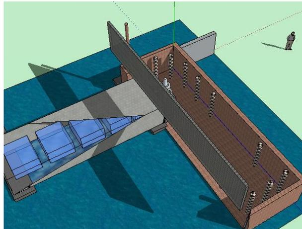
Figure 9- 34. Designed dry chamber for barge gate when not in operation
