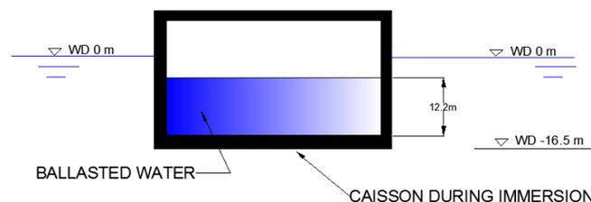
Figure 9- 18. Caisson during immersion to WD-16.5m at final location
