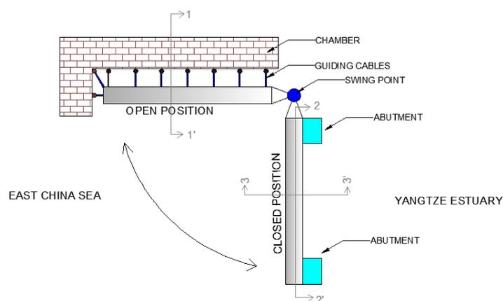
Figure 9- 2. Plan view of the floating barge gate, not to scale (not to scale)
