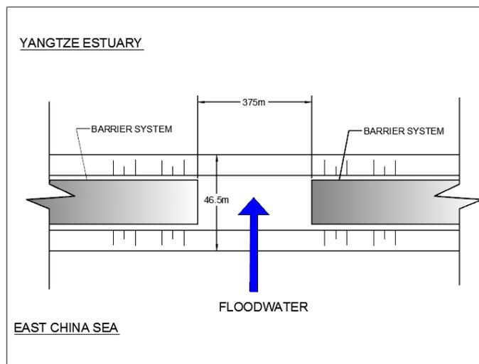
Figure 10- 8. Flow through opening during floods
