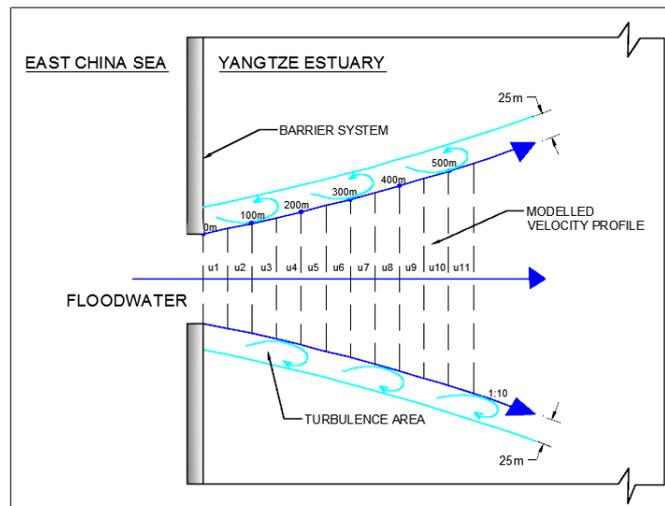
Figure 10- 7. Modeled discrete velocity profile
