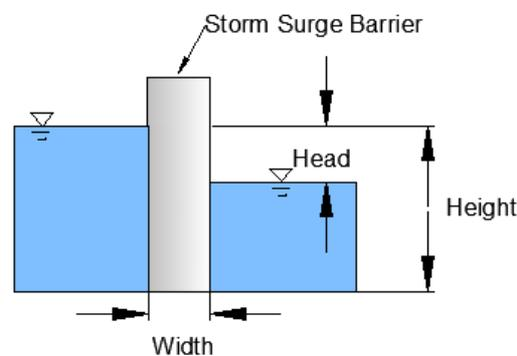
Figure E- 1. Simplified Storm Surge Barrier Cross Section
