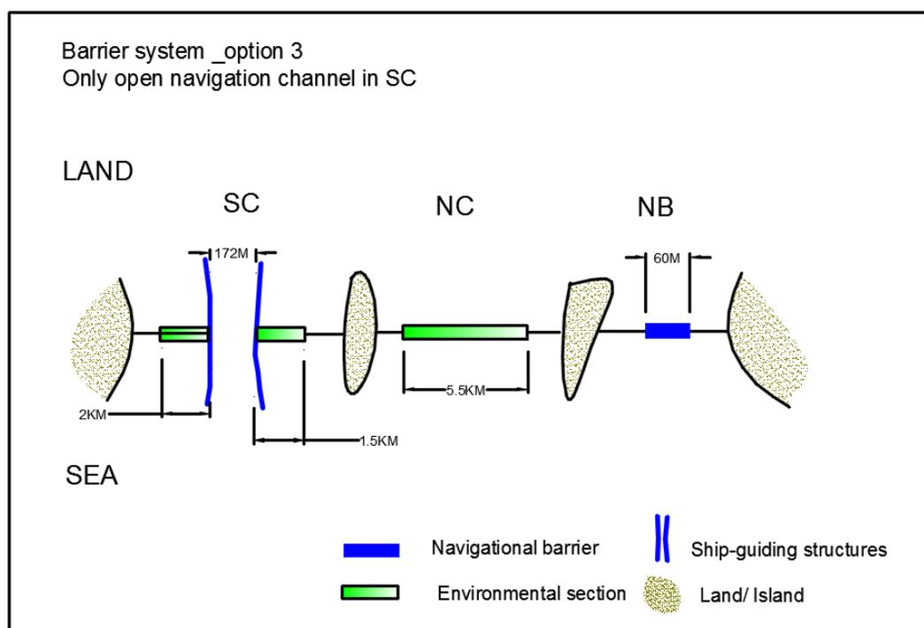
Figure 10- 1. Schematic plan view of open option
