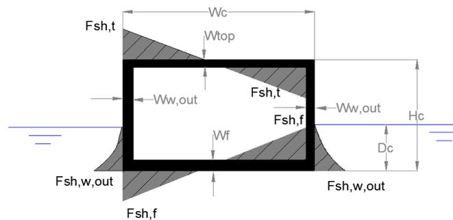
Figure 9- 14. Shear stress scheme on a floating caisson
