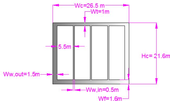
**Figure 9- 12. Initial compartment dimensions in the width direction**
