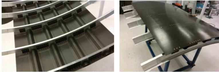
Figure 3.1: Stiffened panel of structural application [43]
