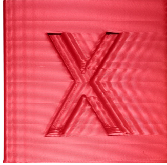
Figure 1.2: Due to the limited stiffness of the belt of a belt-driven system, vibrations and belt stretch cause ringing in the final manufactured product. A similar effect is seen in laser cutting machines [31].
