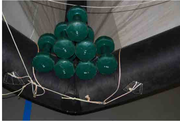
Figure 8-5: Kite under gravity and center load
