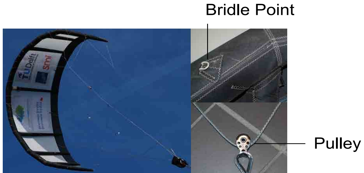
Figure 2-15: Bridle system, pulleys knots and bridle point
