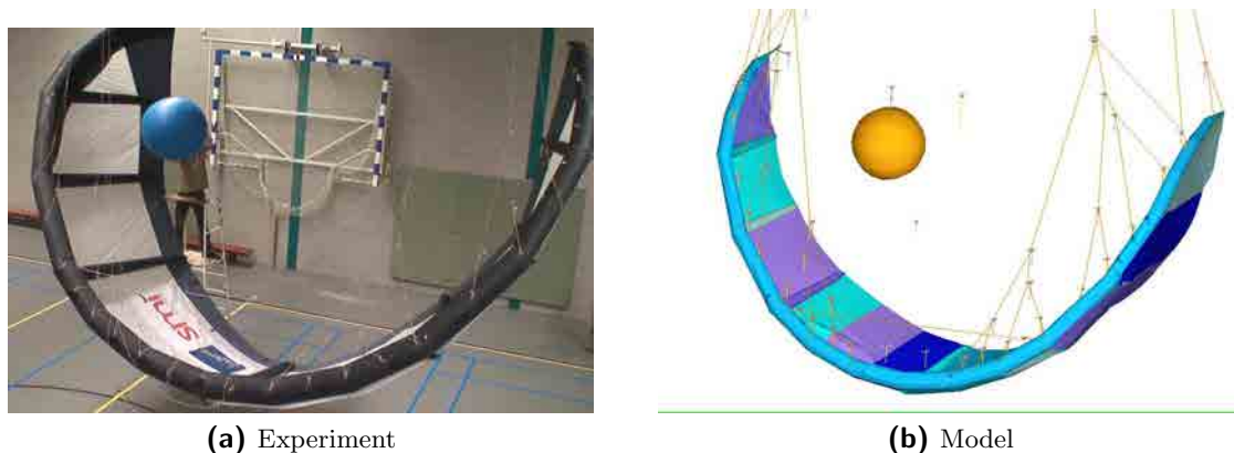
Figure 8-25: Falling mass comparison t = 0 s
