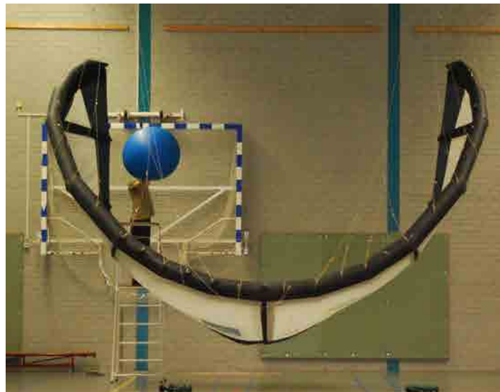
Figure 8-6: Dynamic interactive test between the kite and a mass
