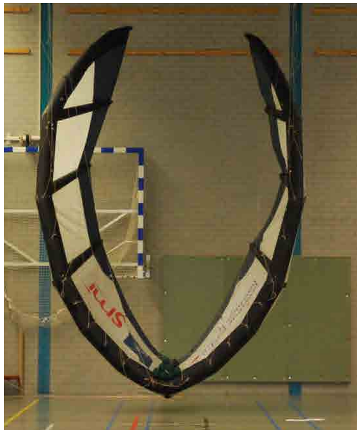
Figure 8-4: Kite under gravity and center load
