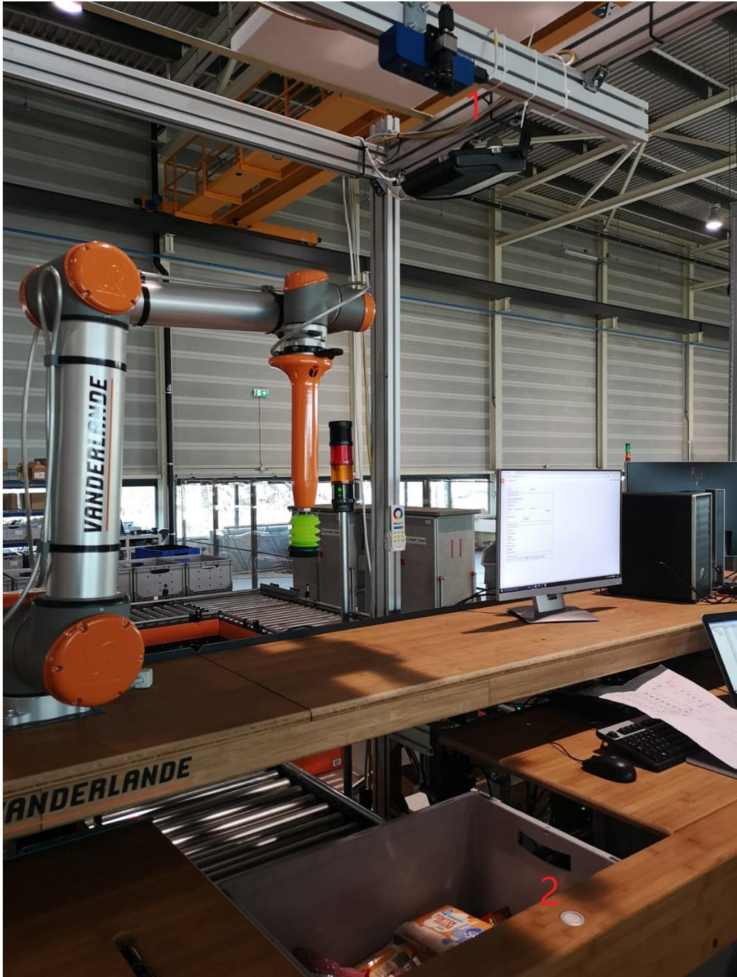
**Figure 3-1:** The camera setup used to capture the data. 1: the dual camera setup, the blue camera being the Ensenso camera for depth images, the black camera being the iDS camera for RGB images. 2: the box with the products inside.
