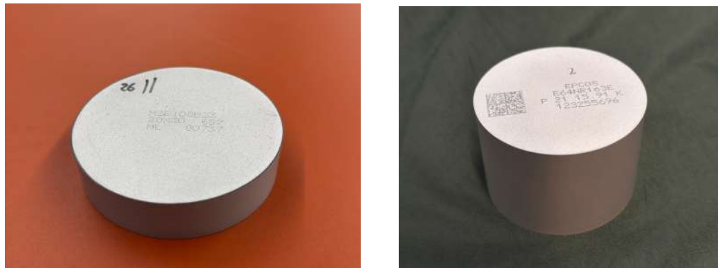
Figure 3. MOV blocks (no.1 left, no.2 right) considered in the study
