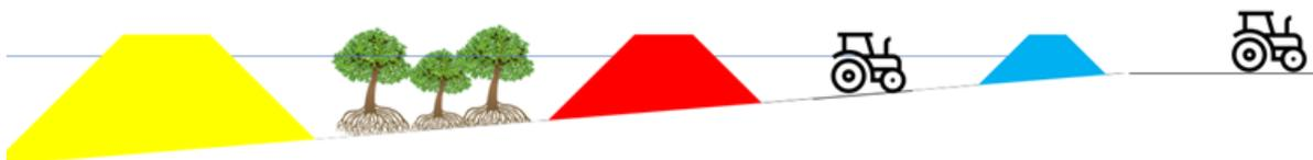
Figure 7.6: Three locations to build a levee. The colors of the levees correspond to those in Figure 7.5. The yellow levee does not allow mangroves to grow. The red levee receives protection from mangroves. The blue option is protected by mangroves and is positioned higher, such that a smaller levee suffices and it is more resilient to sea level rise. However, the agricultural land in front of the blue levee is lost due to salinization.
