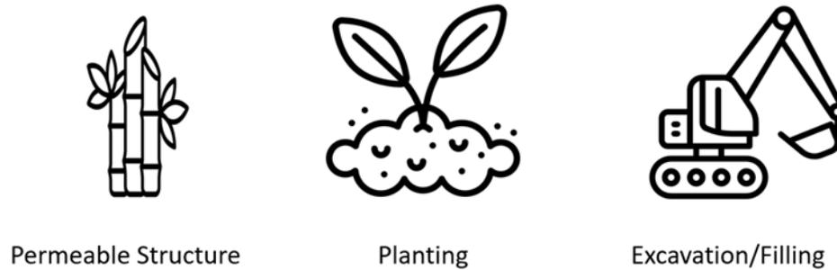
Figure 2.2: Mangrove restoration options can be segmented into three main options: building a permeable structure, planting mangroves and hydrologic restoration in the form of excavation/filling. A permeable structure can be in the form of a bamboo fence and reduces wave energy such that mangroves are able to grow again. For planting mangroves mainly seedlings or propagules are used.
