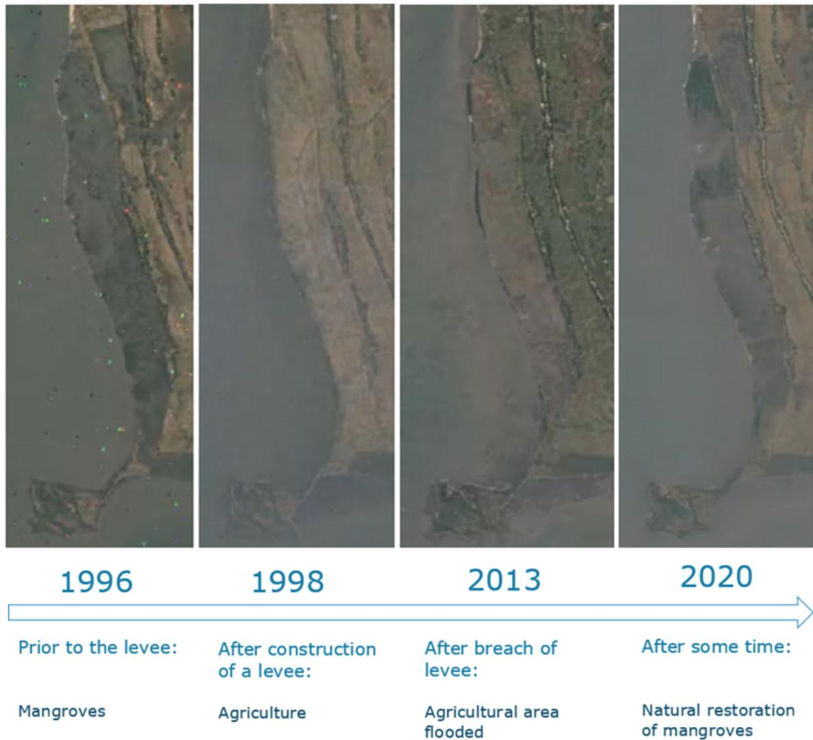
Figure 7.1: Timeline of the situation at the coast of Kaback. In 1996, a mangrove forest was present. After building a levee in 1997, the mangroves disappeared. After the levee breached in 2012, the agricultural area flooded and mangroves grew back naturally.
