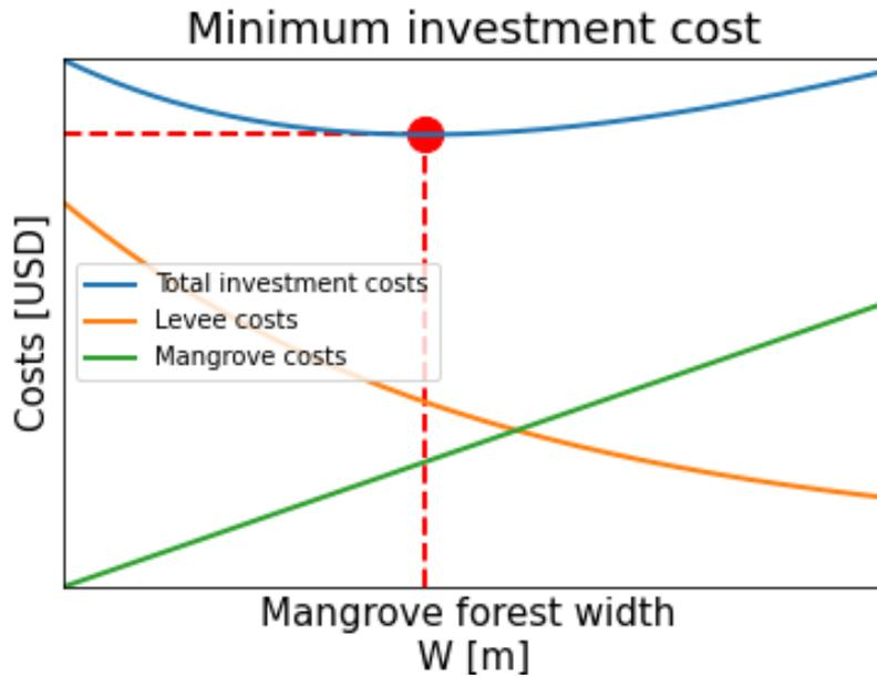
Figure 4.3: The essence of the model is to minimize investment costs by finding the optimal combination of levee and mangroves for a given safety level. A wider mangrove forest reduces the required height of the levee.
