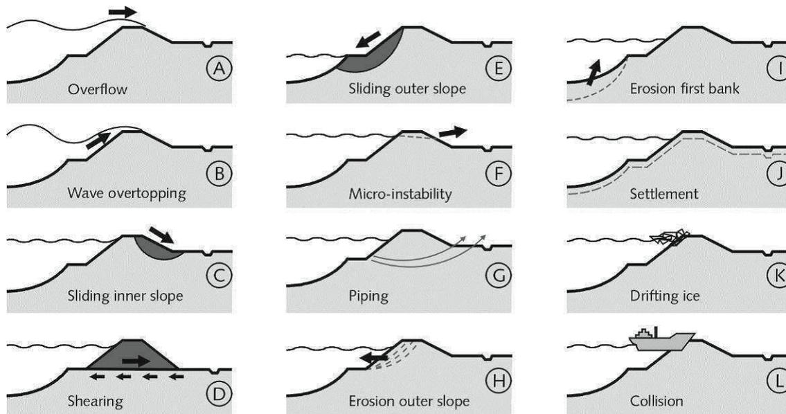
Figure 2.5: Possible failure mechanisms (Jonkman et al., 2020). This thesis focuses on the failure mechanism of wave overtopping (B). Failure occurs if the discharge of water over the levee is higher than the critical discharge for which the levee fails.
