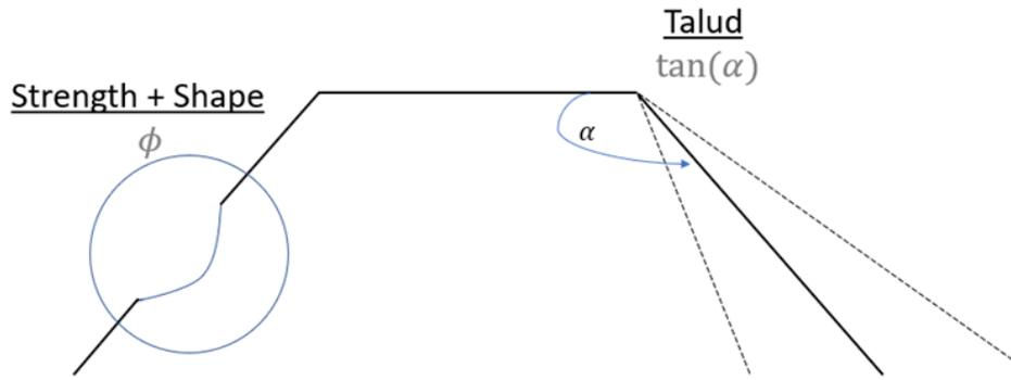
Figure 4.5: Maximum wave overtopping and therefore maximum wave run-up depends on the shape and strength of the levee.  $\phi$  represents the shape and strength of the levee (Van der Meer et al., 2016), while  $\tan(\alpha)$  represents the talud of the levee. These are design choices and may affect the costs of the levee. In this thesis,  $\phi = 8$  is applied based on Van der Meer et al. (2016) and  $\tan(\alpha) = 0.25$ .
