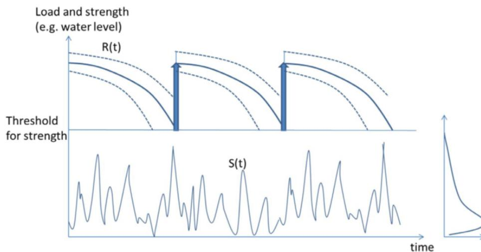
Figure 2.4: Load and strength of a levee schematized over time. Figure copied from Jonkman et al. (2018).
