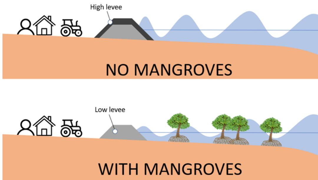
Figure 4.2: Sketch of the situation with and without mangroves. Without mangroves, the wave is not attenuated by vegetation: the levee has to withstand the unaffected wave run-up. With mangroves, the wave height is attenuated, reducing the wave run-up and as a result a lower levee height suffices.
