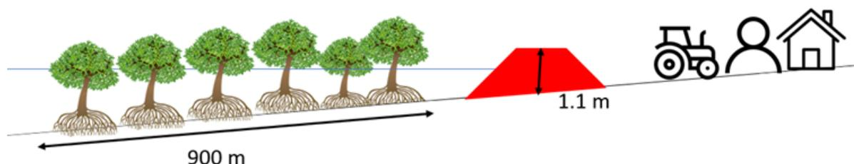
Figure 7.10: Schematization of the optimal solution for Kaback. A levee just behind the mangroves of 1.1 m combined with a mangrove forest of 900 m is optimal.
