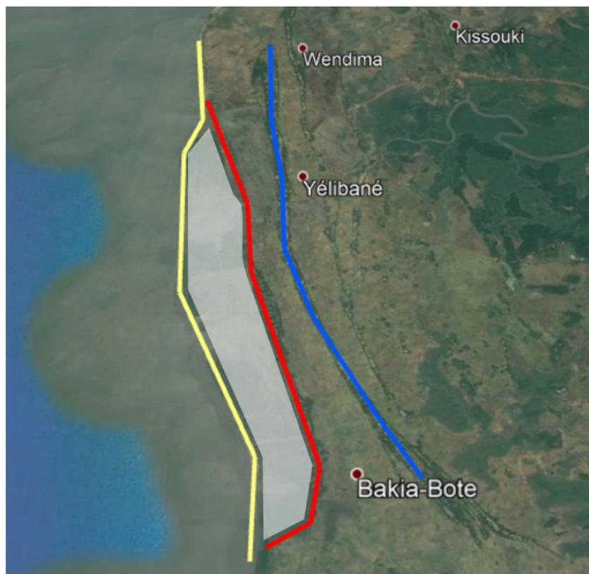
Figure 7.5: Three possible positions of a levee as indicated by the colored lines. **yellow** = in front of the mangroves, **red** = just behind the mangroves, **blue** = land inwards. The white shaded area represents the area where mangroves can grow.
