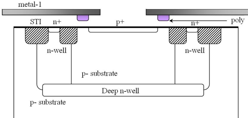
**Figure 4.32:** Cross-section of LDD guard ring based structures integrated in 65nm CMOS technology.
