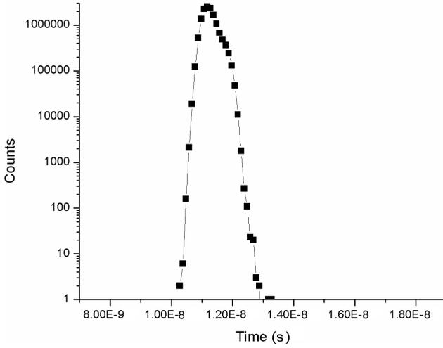
**Figure 4.24:** Histogram of the time between the laser pulse and the SPAD receiving digital pulse at 405nm wavelength.
