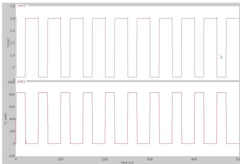
**Figure 4.42:** *The transient time simulation of the capacitance part voltage convertor.*
