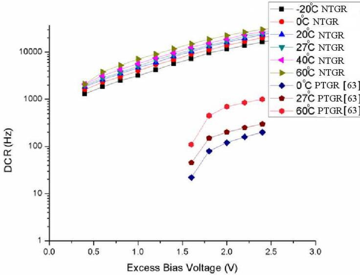
**Figure 3.11:** DCR behavior at different excess bias voltages as a function of temperature.
