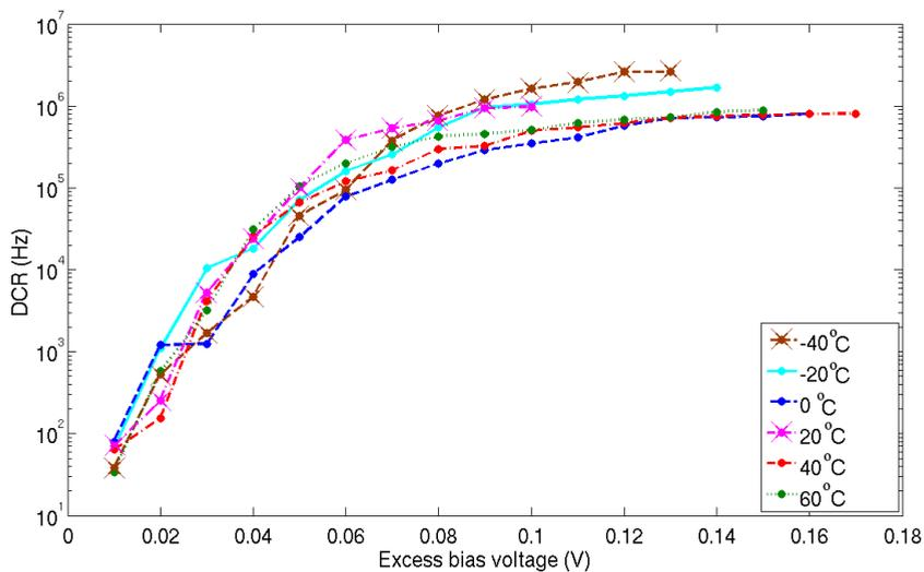
**Figure 4.11:** DCR of the first sub-family of SPADs in 90nm technology at different excess bias voltages and different temperatures. (All the SPADs are based on n-well guard rings).
