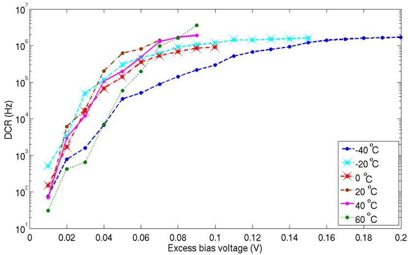
**Figure 4.13:** DCR of the third group of SPADs in 90nm technology at different excess bias voltages and different temperatures. (All the SPADs are based on n-well guard rings).
