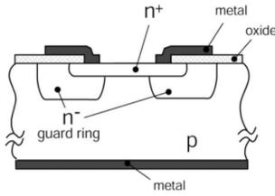
**Figure 2.2:** *Haitz's APD using diffused guard ring as the first planar devices proposed as SPAD [20].*
