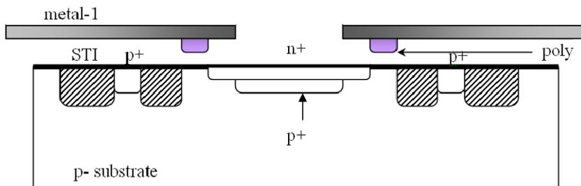
**Figure 4.35:** *Cross-section of the proposed structure based on an enrichment  $p^+$  region.*
