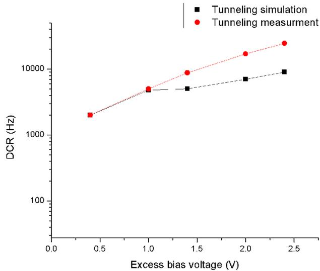
**Figure 3.10:** Comparison of theoretical model and measurement of DCR for NTGR SPAD at different excess bias voltages.
