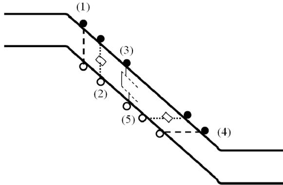
**Figure 2.10:** Generation mechanisms in a SPAD (1) Thermal direct generation (2) SRH trap-assisted generation (3) Excitonic generation (4) Band-to-band tunneling (5) Trap-assisted tunneling.
