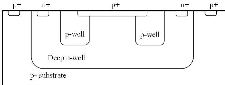
**Figure 3.19:** *Cross-section of a SPAD implemented in  $0.8 \mu\text{m}$  CMOS process.*
