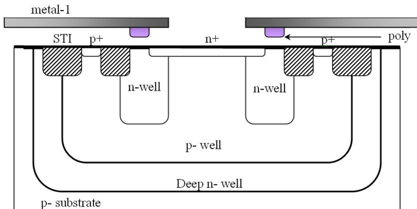
**Figure 4.17:** *Eliminating coupling between SPAD and substrate using deep n-well and p-well.*
