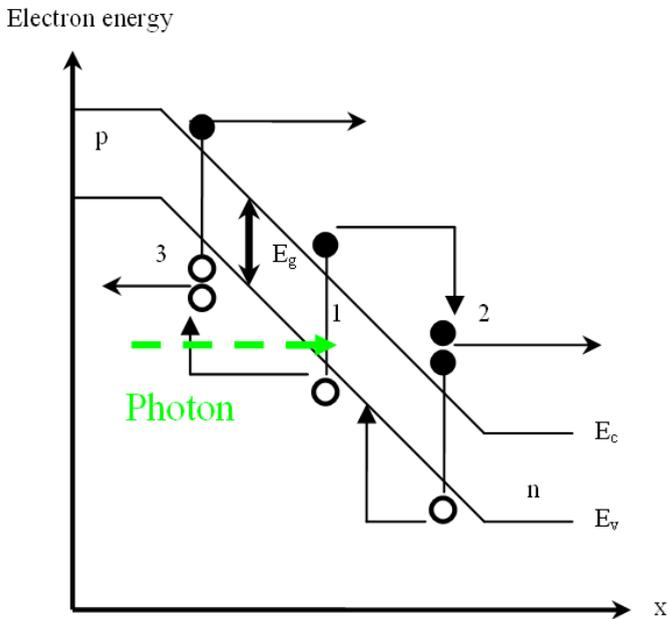
**Figure 1.5:** The multiplication process in an APD.
