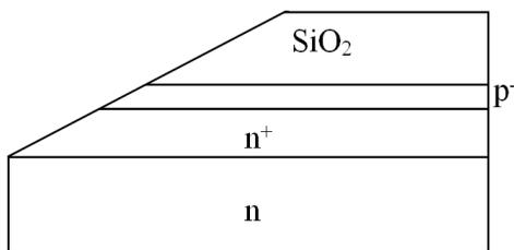
**Figure 2.6:** *Beveled junction. The depletion region is between  $n^+$ , and  $p^-$  [30].*
