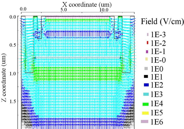
**Figure 4.34:** Electric field simulation of LDD guard ring based structure at room temperature.
