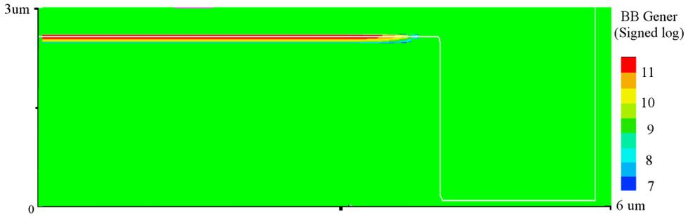
**Figure 3.6:** *Contours of BTBT generation rate in NTGR SPAD. The picture shows a half of the cross-section of the SPAD.*
