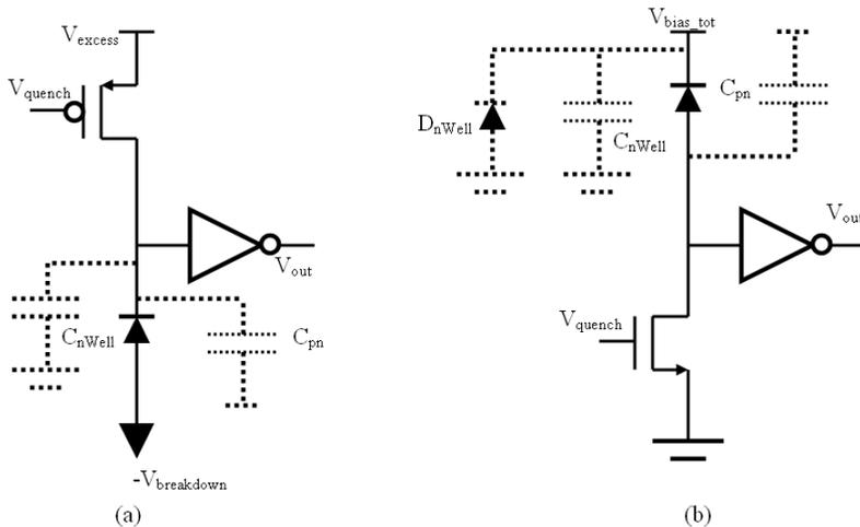
**Figure 4.39:** SPAD biasing options (a) cathode (b) anode, as the reference for output signal.
