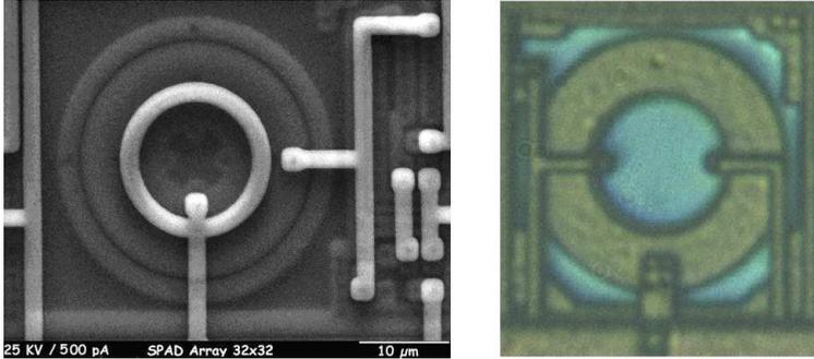
**Figure 3.20:** Scanning Electron Microscope (SEM) image of a SPAD implemented in  $0.8\ \mu\text{m}$  CMOS process, and photomicrograph of a SPAD implemented in  $0.35\ \mu\text{m}$  CMOS process which shows the RTS behavior after irradiation.
