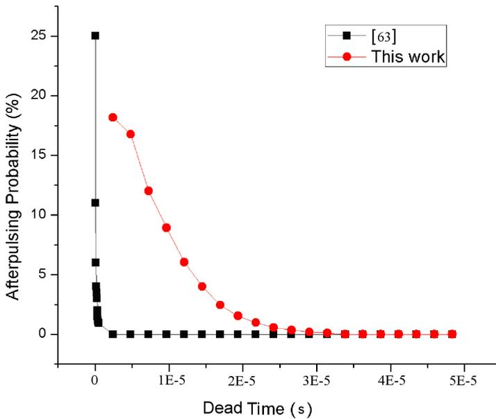
**Figure 3.14:** *Afterpulsing probability of NTGR SPAD vs dead time.*
