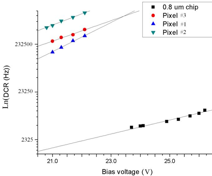
**Figure 3.31:** DCR RTS amplitude vs bias voltage at room temperature. The fitting function is  $y = ae^{bx}$ , where  $a$ , and  $b$  are equal to 0.5783, and 0.336 for 0.8 $\mu\text{m}$  chip, 3.52, and 0.4954 for pixel No.3, 0.026, and 0.704 for pixel No.1, and 2.89, and 0.541 for pixel No.2.
