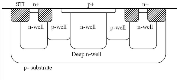
**Figure 2.13:** *Retrograde doping introduction for jitter reduction in SPADs.*
