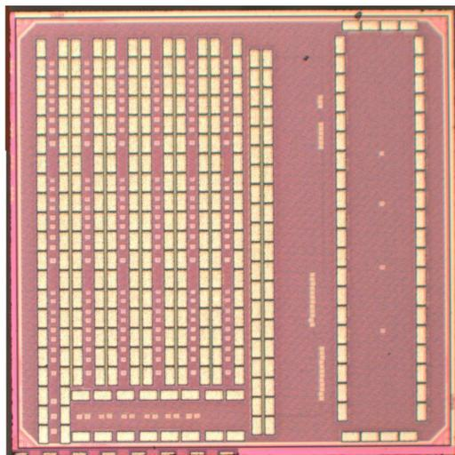
**Figure 4.9:** Photomicrograph of the SPAD farm.
