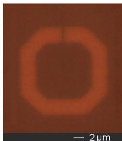
**Figure 4.14:** Photomicrograph of an octagonal SPAD. The guard ring is covered with metal to prevent light absorption in the guard ring region.
