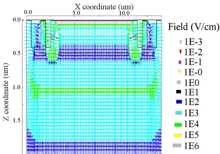
**Figure 4.30:** Electric field simulation result of low voltage p-well guard ring SPAD at room temperature.
