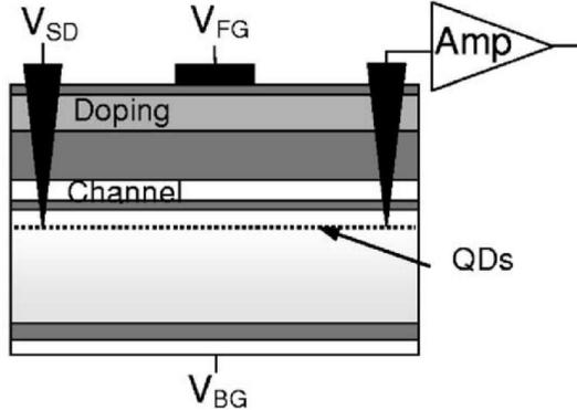
**Figure 1.7:** Schematic of a quantum dot single-photon detector [9].
