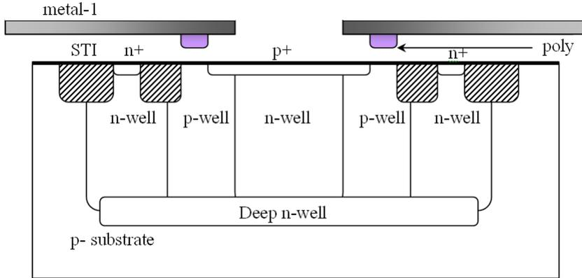
**Figure 4.1:** Cross-section of the p-well based guard ring SPAD in 90nm CMOS technology.
