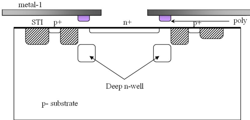
**Figure 4.27:** Cross-section of deep n-well guard ring SPAD integrated in 65nm technology.
