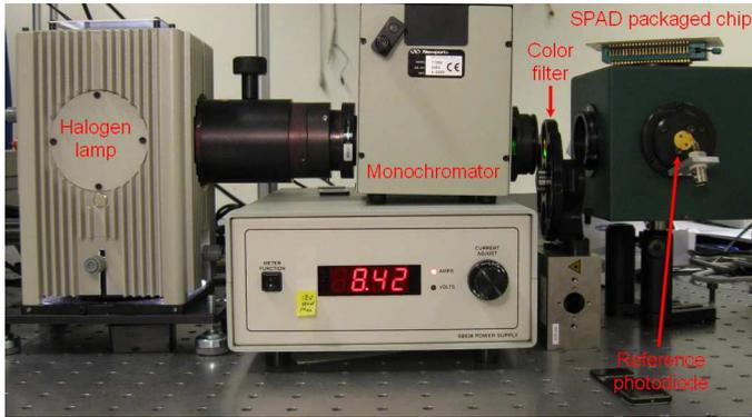
Figure 4.22: Optical setup for PDP measurement.
