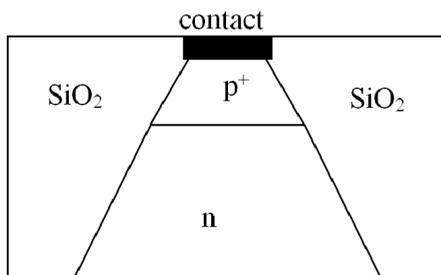
**Figure 2.7:** *Mesa isolation as the guard ring of SPAD [5].*
