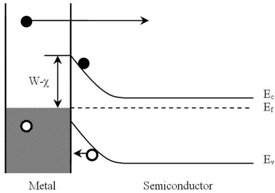
**Figure 1.4:** Energy band diagram of a Schottky-barrier photodiode formed by depositing a metal on a n-type semiconductor. This photodetector is responsive to the photon energies larger than the Schottky barrier height  $h\nu > W - \chi$ .
