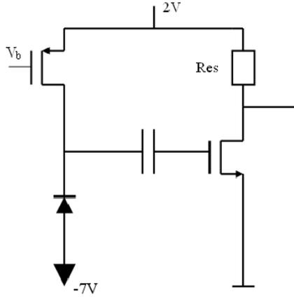
**Figure 4.40:** Implemented circuit for digitalizing the SPAD output.
