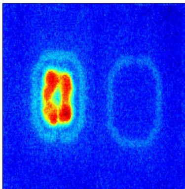
**Figure 4.26:** *Photoluminescence of a SPAD operating in Geiger and sub-Geiger mode.*
