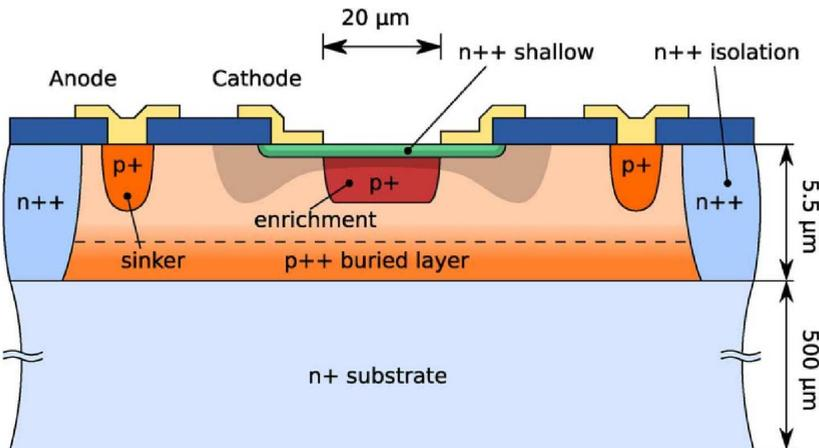
**Figure 2.3:** *Cross-section of double-epitaxy SPAD [23].*
