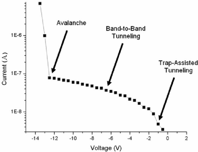
**Figure 3.5:** *I-V characteristic of a SPAD implemented in 0.35  $\mu\text{m}$  technology.*
