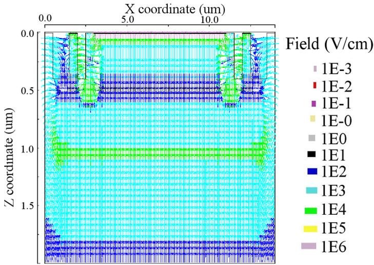
**Figure 4.33:** Electric field simulation result of the STI-bound p-substrate guard ring SPAD at room temperature.
