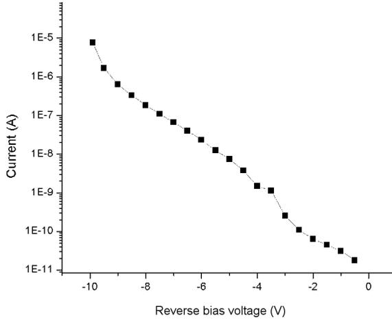
**Figure 4.6:** *I-V characteristic of the p-substrate guard ring based SPAD in 90nm technology.*
