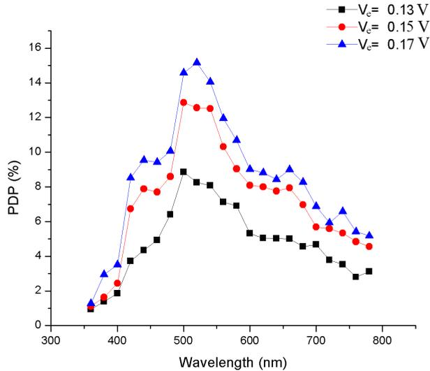
**Figure 4.23:** *Photon Detection Probability (PDP) of a SPAD implemented in 90nm technology. The PDP was measured with a monochromator and reference photodetector at room temperature.*
