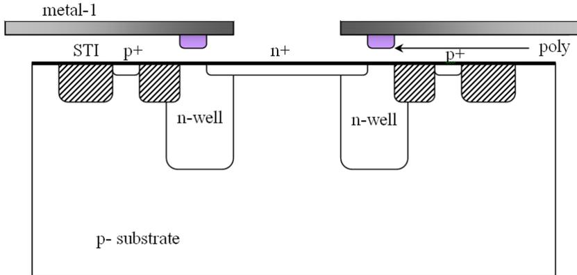
**Figure 4.7:** *Cross-section of n-well based guard ring SPADs in 90nm technology.*
