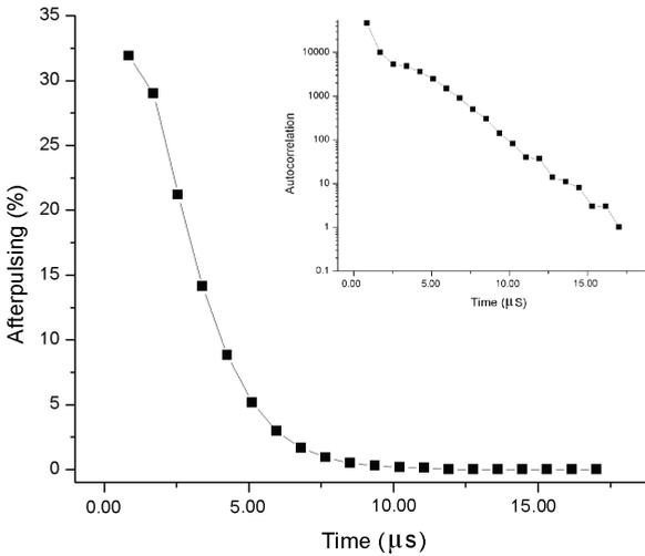
**Figure 4.25:** Afterpulse probability as a function of dead time. In the inset the corresponding autocorrelation function.
