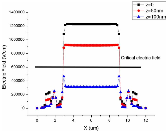
**Figure 4.16:** *Electric field strength in the cross-section of the SPAD at different depths.*
