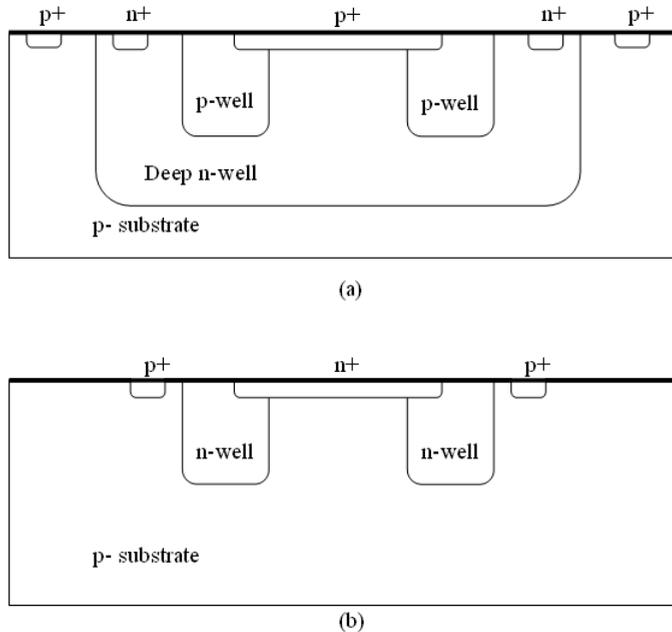
**Figure 3.4:** Cross-section of a p-tub guard ring (PTGR) SPAD (a), and a n-tub guard ring (NTGR) SPAD (b).
