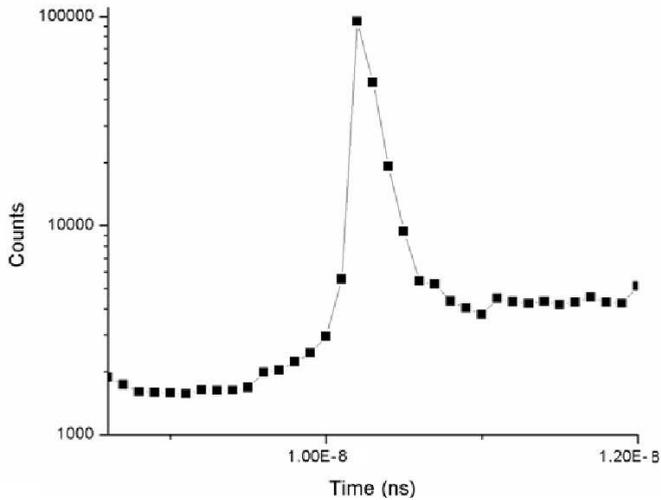
**Figure 3.13:** Output signal of a SPAD exposed to 40 MHz pulsed laser for jitter measurements at 405 nm wavelength at room temperature.
