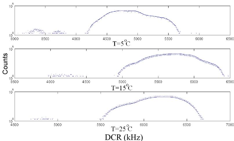
**Figure 3.27:** DCR histogram of a pixel: DCR levels number decreasing vs temperature.
