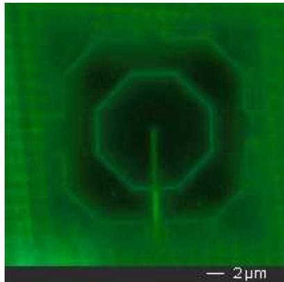
Figure 4.38: Photomicrograph of an octagonal SPAD implemented in 65nm technology. The guard ring is covered with metal to prevent light absorption in the guard ring region.
