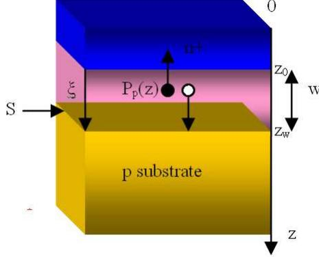
**Figure 3.3:** Main elements for tunneling integral calculation in junction cross-section.
