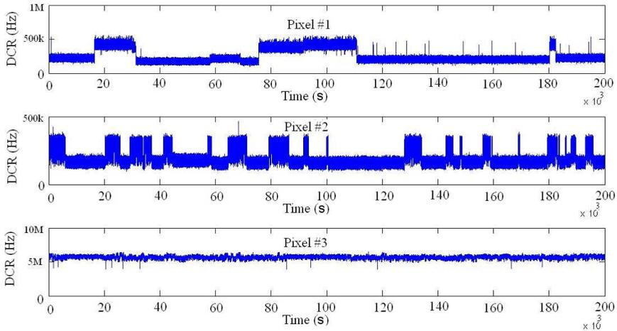
**Figure 3.23:** *Different forms of RTS in 3 pixels of a proton irradiated SPAD.*
