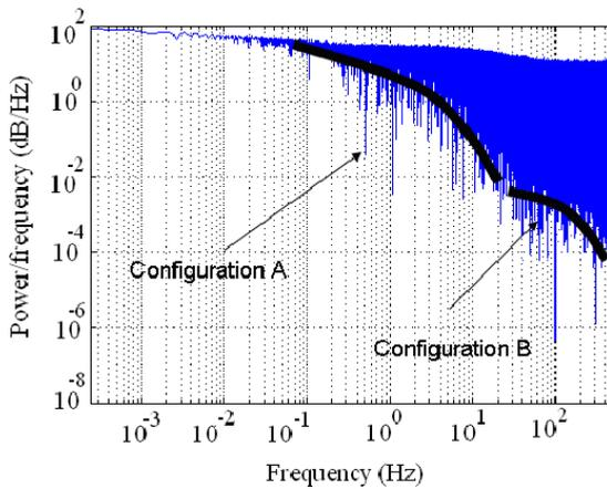
**Figure 3.25:** Different configurations of the traps or defects effects in the power spectral density of the DCR.
