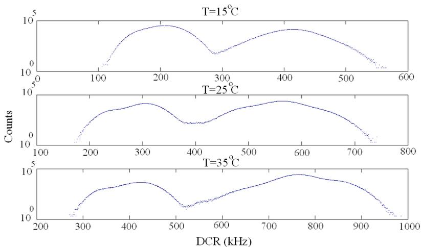
**Figure 3.28:** DCR histogram of another pixel: An increase in DCR levels number in temperature.
