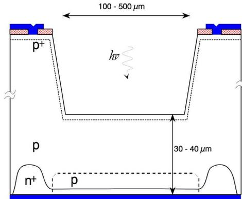
**Figure 2.1:** *Reach-through Single-photon detector. The device contains different absorption and multiplication regions [15].*
