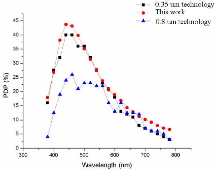
**Figure 3.12:** Photon detection probability of NTGR SPAD at different wavelengths.
