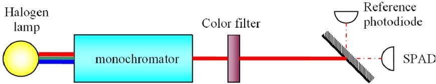
Figure 4.21: Schematic configuration of PDP measurement setup.
