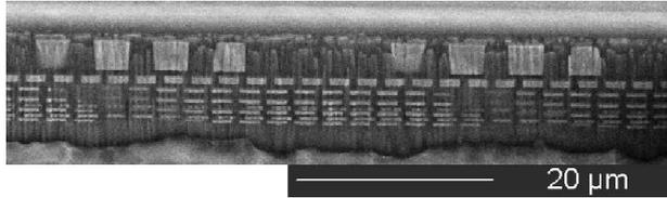
**Figure 2.11:** *Scanning Electron Microscopy of optical stacks in 90nm CMOS technology. The optical stack consists of 9 metal layers and 7 passivation layers decreasing the photon absorption.*
