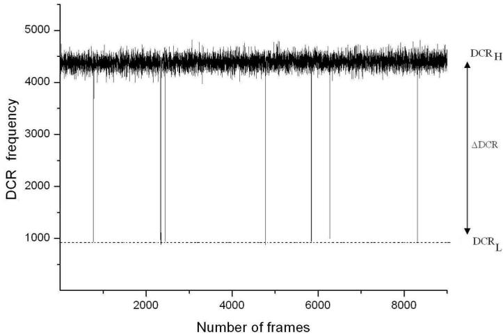
**Figure 3.22:** *Bistable DCR levels in  $0.8\mu\text{m}$  CMOS non-irradiated SPAD.*
