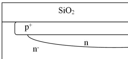
**Figure 2.8:** *Straddled junction as the guard ring for SPADs [5].*
