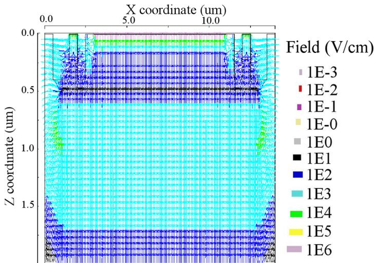
**Figure 4.5:** Spectra simulation of the electric field distribution of the p-substrate guard ring based SPAD in 90nm technology.
