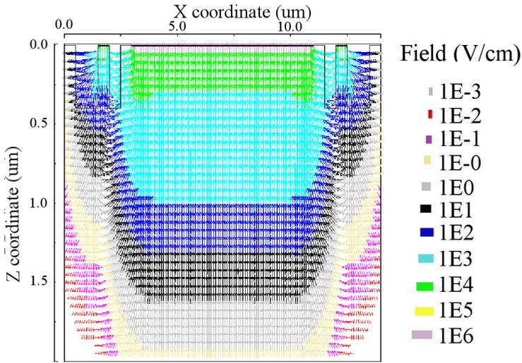
Figure 4.37: Electric field simulation of the SPAD structure at room temperature.
