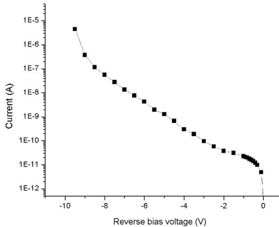
**Figure 4.2:**  $I$ - $V$  characteristic of the p-well guard ring based SPAD.
