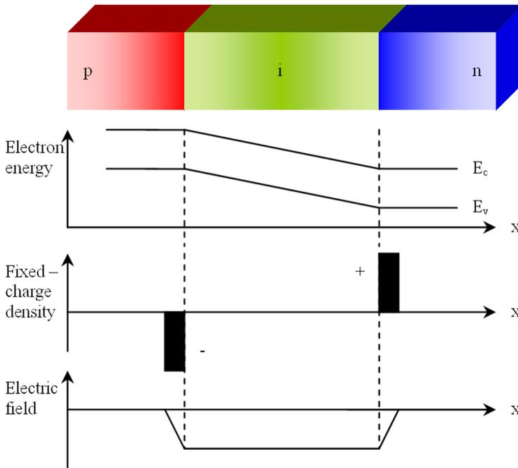
**Figure 1.3:** The  $p-i-n$  energy diagram, charge distribution and electric field distribution. The device can be illuminated parallel to the junction or perpendicular.
