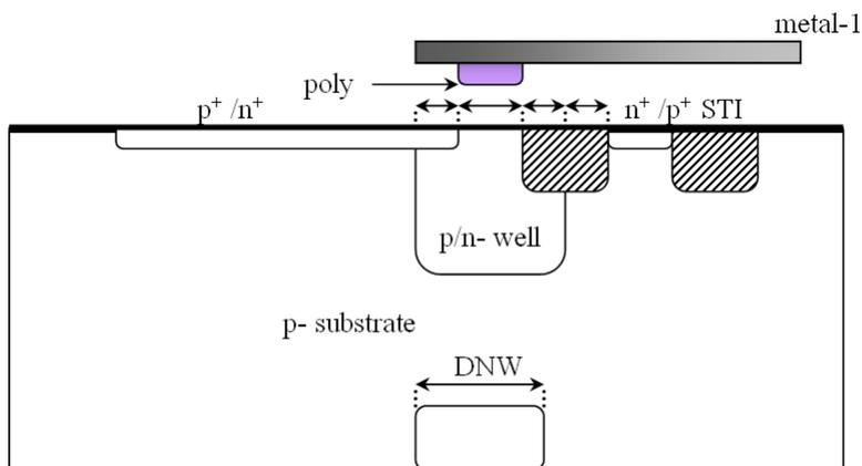
**Figure 4.36:** *The Five main parameters varied in each family of SPAD: poly width, extension of p/n+ in guard ring and extension of STI in the guard ring, STI overlap with p/n-wells, and the Deep n-well width.*
