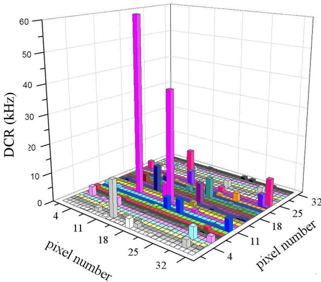
**Figure 3.21:** DCR distribution among the pixels of the  $32\times 32$  SPAD array.
