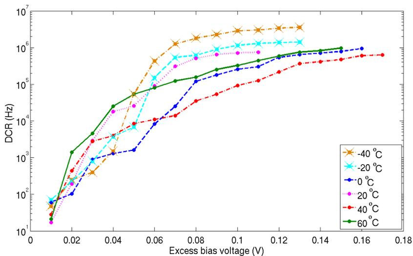
**Figure 4.12:** DCR of the second sub-family of SPADs in 90nm technology at different excess bias voltages and different temperatures. (All the SPADs are based on n-well guard rings).
