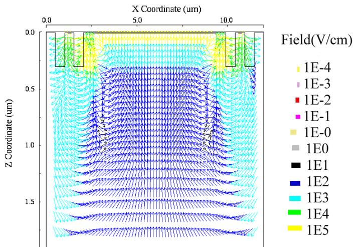
**Figure 4.15:** Electric field distribution of the n-well guard ring based SPAD in 90nm technology, biased above breakdown.
