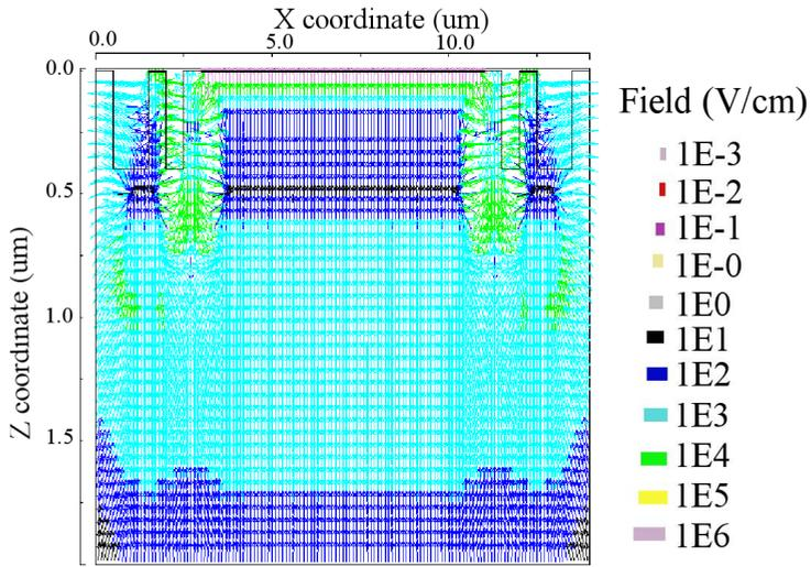
**Figure 4.4:** Electric field distribution on the p-well guard ring based SPAD.
