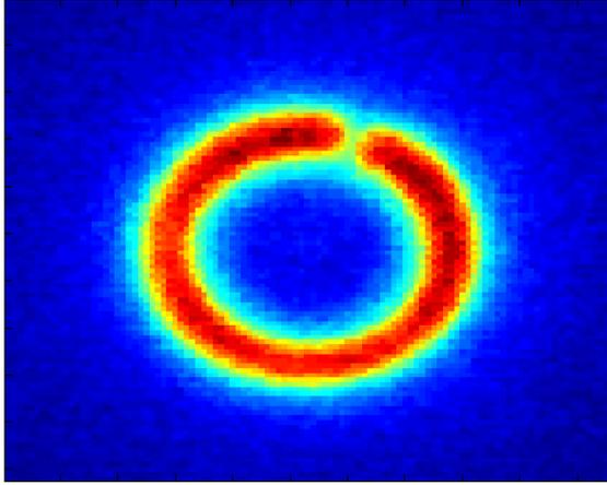
**Figure 3.15:** *Photoemission of a non-functional NTGR SPAD. The figure shows the light emission from the guard ring due to PEB.*
