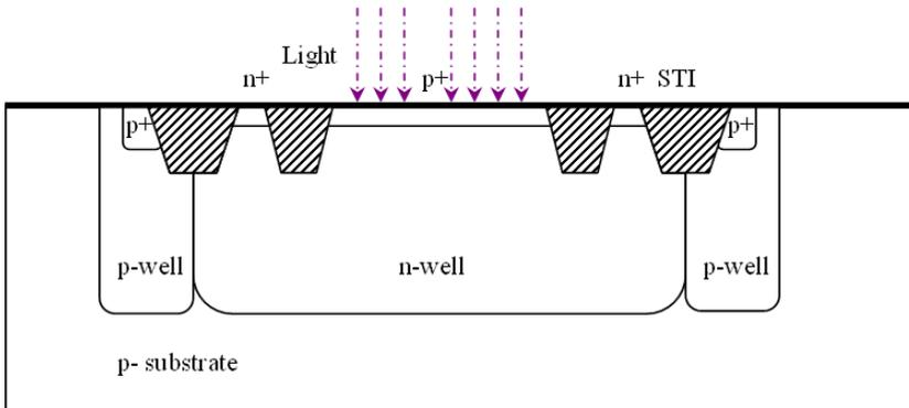
**Figure 2.5:** *Cross-section of SPAD using STI layer as guard ring.*
