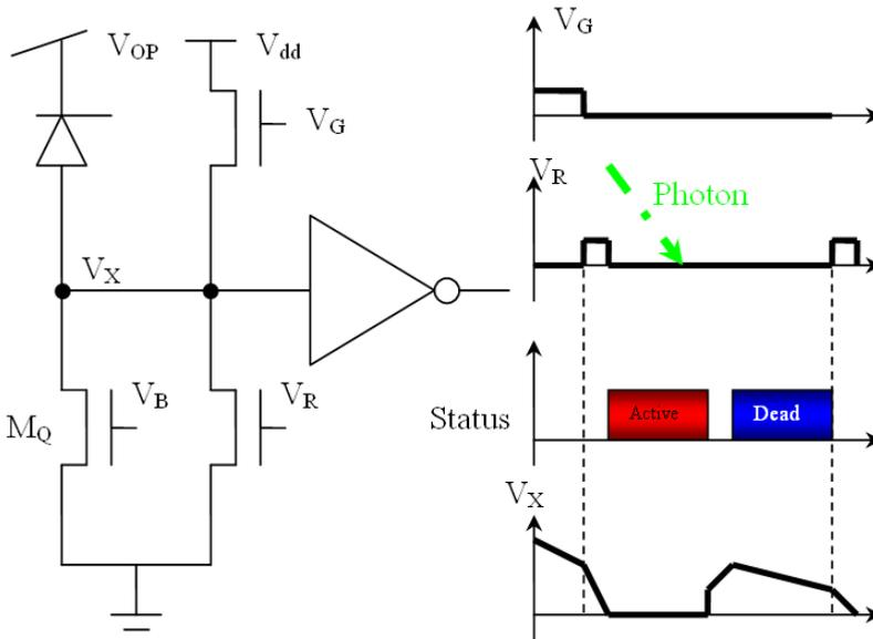
**Figure 1.9:** Active circuit for gating and quenching of SPAD.
