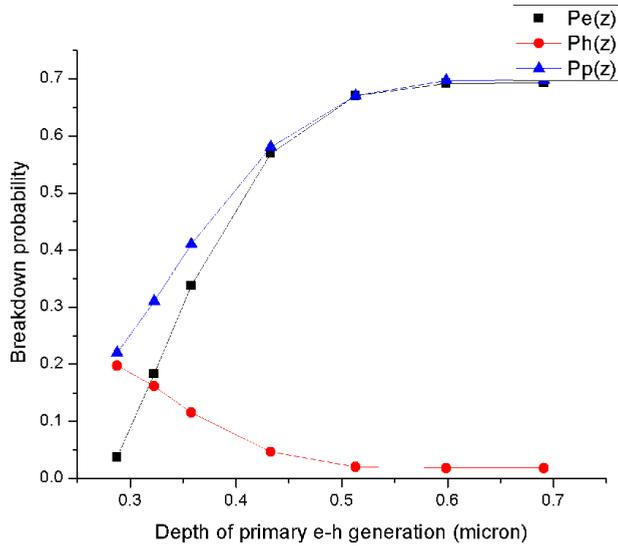
**Figure 3.9:**  $P_e(z)$ ,  $P_h(z)$ , and  $P_p(z)$  at different depths. Avalanche trigger probabilities calculated for NTGR SPADs at 1.4 Volts of excess bias voltage.  $z$  is the same as Figure 3.3.
