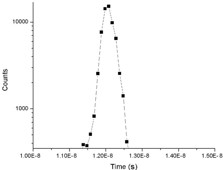
**Figure 2.12:** *Timing histogram of a SPAD, representing 368 ps FWHM jitter.*
