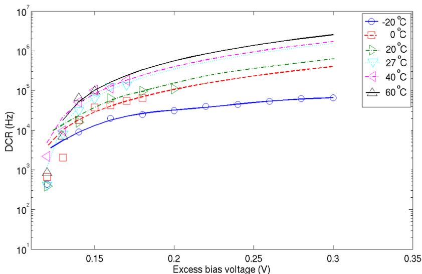
**Figure 4.20:** *DCR vs. excess bias voltage for different temperatures. The curves were fitted to show the trend of DCR in different biasing conditions.*
