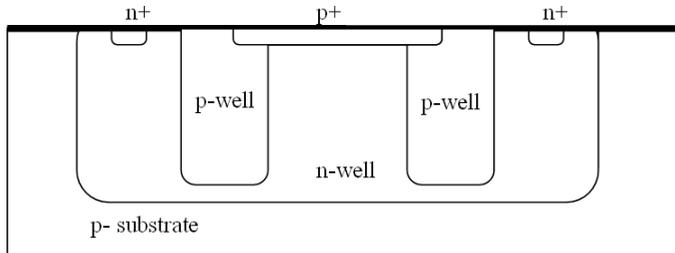
**Figure 2.4:** *Cross-section of a standard CMOS SPAD proposed by Rochas.*
