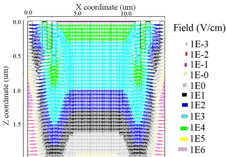
**Figure 4.29:** Electric field simulation result of deep n-well guard ring based SPAD at room temperature. The critical electric field for impact ionization is  $6 \times 10^5 \text{V/cm}$  in silicon.
