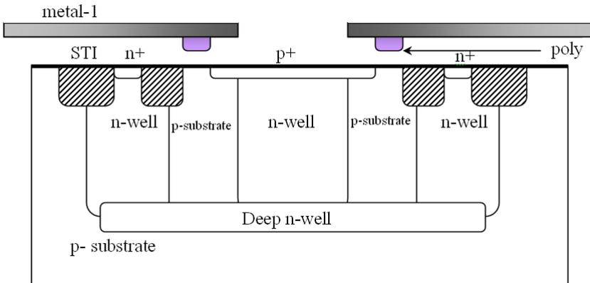
**Figure 4.3:** Cross-section of p-substrate based guard ring SPAD in 90nm technology.
