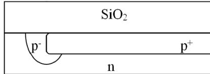
Figure 2.9: Diffused guard ring as guard ring of SPAD [34].
