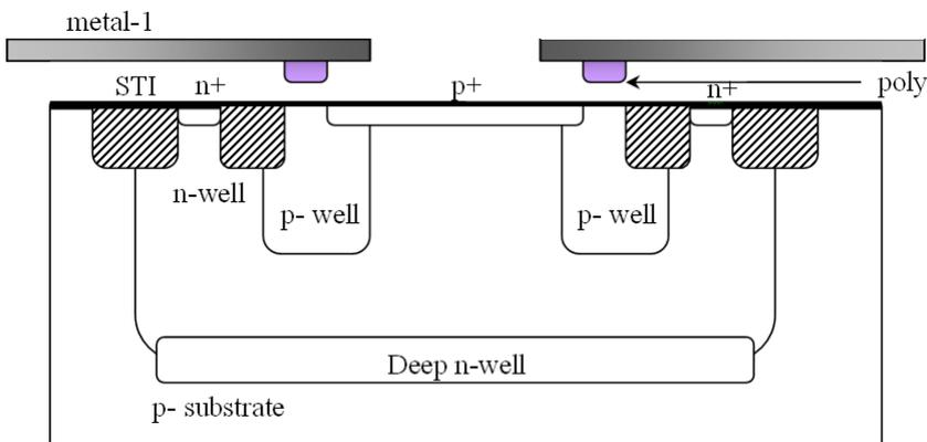
**Figure 4.28:** Cross-section of low voltage p-well guard ring SPADs.
