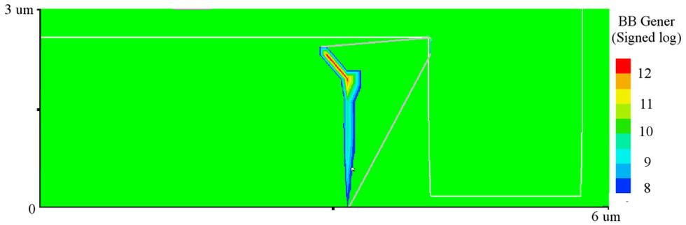
**Figure 3.7:** *Contours of BTBT generation rate in PTGR SPAD. The picture shows a half of the cross-section of SPAD. The inset shows the tunneling profile on the guard ring edge.*
