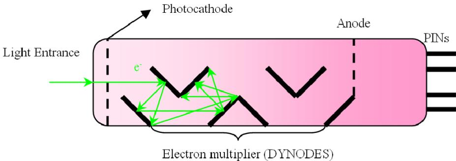
**Figure 1.1:** *Different parts of a photomultiplier tube. The light is generating an electron that will be multiplied in different phases.*
