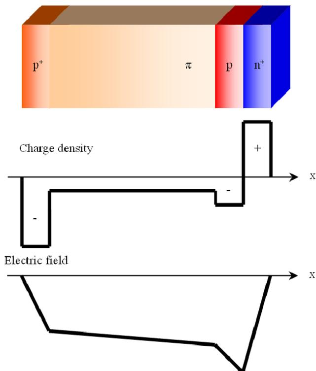
**Figure 1.6:** Reach through  $p^+ - \pi - p - n^+$  APD structure, the charge density distribution and electric field.
