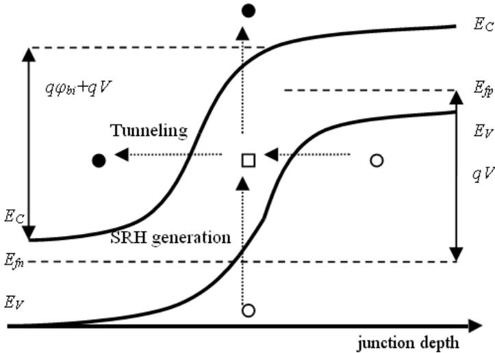
**Figure 3.2:** Mechanisms which a trap can affect SPAD behavior (trap assisted tunneling and trap assisted generation).
