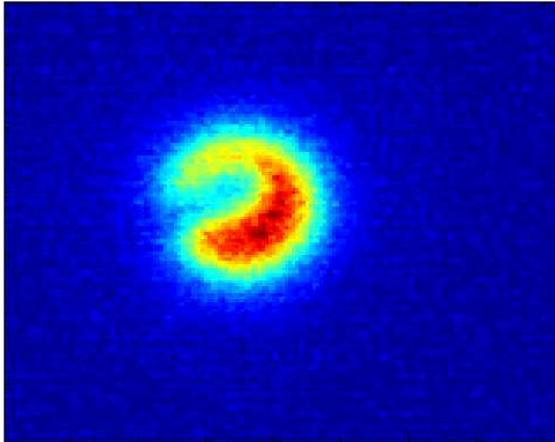
**Figure 3.16:** *Photoemission from the light sensitive area of a working NTGR SPAD. The figure shows virtually no PEB on the guard ring.*
