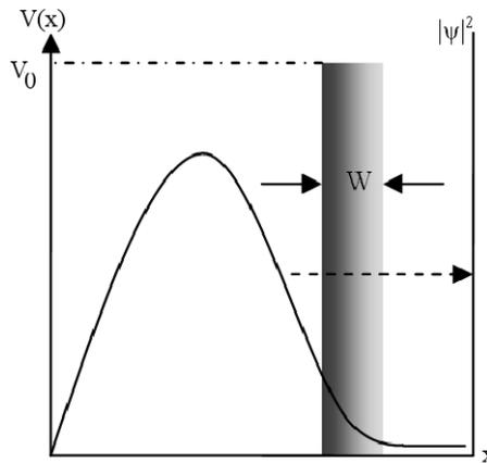
**Figure 3.1:** Tunneling probability vs. depth in quantum wells with finite potential barriers.
