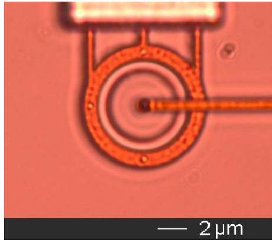
**Figure 3.17:** *Photomicrograph of the circular NTGR SPAD characterized in this section.*
