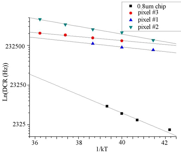
**Figure 3.30:** DCR RTS amplitude vs. temperature in four different pixels at constant excess bias voltage. The fitting function is  $y = ae^bx$ , where  $a$ , and  $b$  are equal to  $3.3e12$ , and  $-0.53$  for  $0.8\mu\text{m}$  chip,  $3.75e5$ , and  $-0.022$  for pixel No.3,  $2.04e7$ , and  $-0.1352$  for pixel No.1, and  $1.92e6$ , and  $-0.05$  for pixel No.2.
