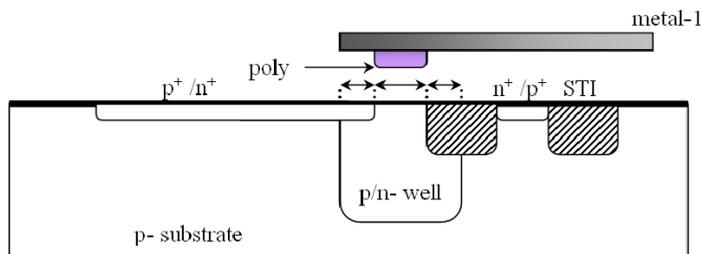
**Figure 4.8:** The three main parameters investigated in each family namely: poly width, extension of p/n+ in guard ring and extension of STI in guard ring.
