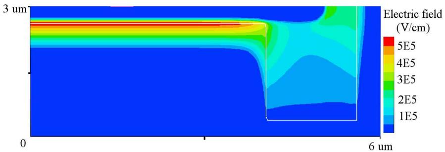
**Figure 3.8:** *Electric field distribution at 1.4 volts of excess bias voltage in NTGR SPAD.*
