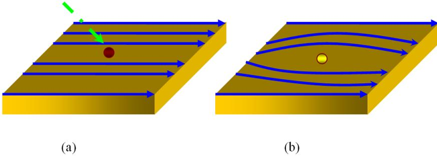
**Figure 1.8:** Operation of a superconducting nanowire photon counter (a) A photon impacts a nanowire carrying a direct current near the critical superconducting current (b) A local hot spot forms, diverting current around it.
