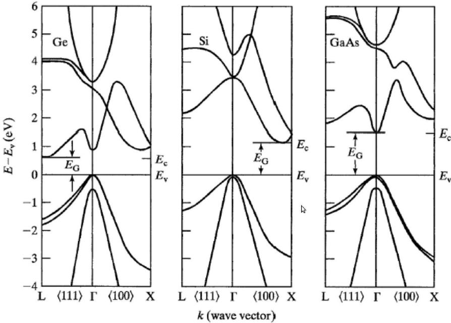
**Figure 3.18:** The energy vs wavevector of indirect (*Si*, *Ge*), and direct (*GaAs*) semiconductors [94].
