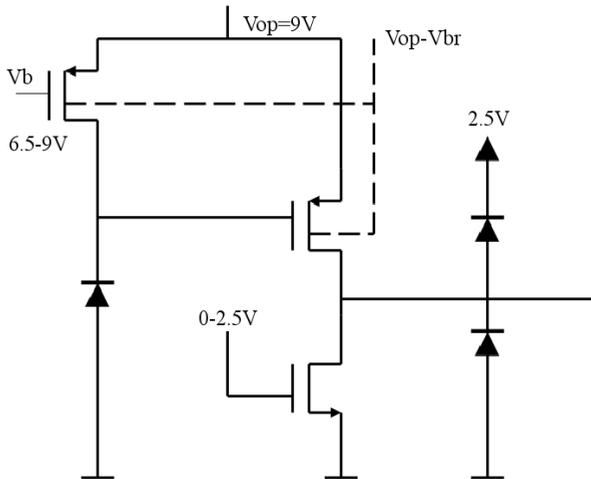
**Figure 4.41:** Second circuit for digitalizing the SPAD output.
