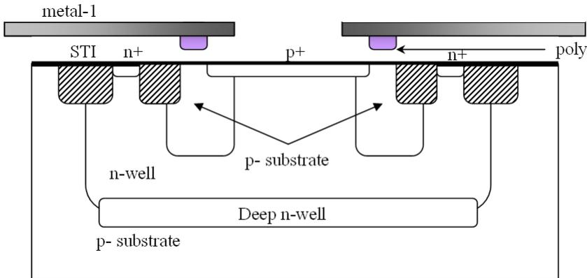
Figure 4.31: Cross-section of STI-bound p-substrate guard ring SPAD.
