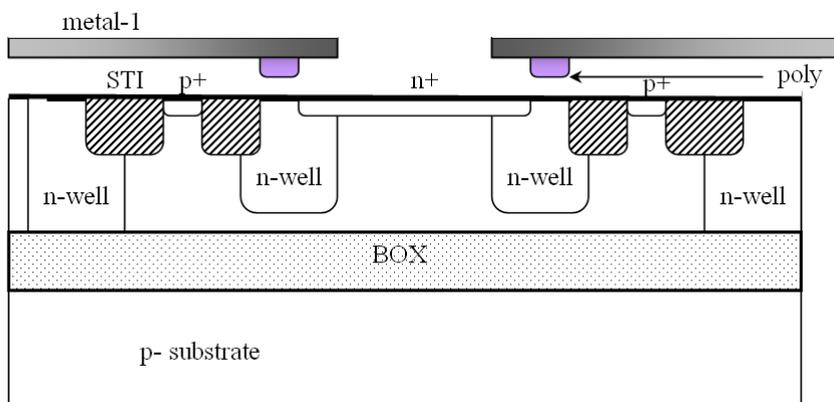
**Figure 4.18:** *Buried oxide layers for eliminating coupling between SOI and substrate.*
