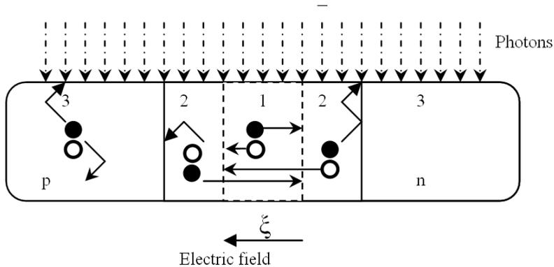
**Figure 1.2:** Cross-section of a  $p-n$  junction showing different regions where the photon can generate an electron-hole pair, and the direction each carrier takes.
