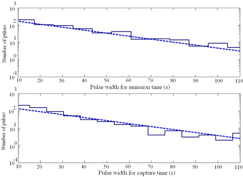
**Figure 3.24:** Pulse width histograms obtained by sorting and counting the capture and emission times of a bistable pixel at room temperature for 8hrs. Dashed lines are the expected number of pulses estimated by equation (3.14).
