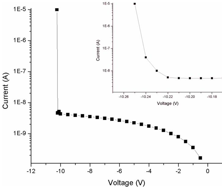
**Figure 4.19:** The I-V characteristic of the diode implemented in 90nm technology which shows photon counting capability. The sharp transition between the band-to-band tunneling region and the avalanche region makes the SPAD suitable for the Geiger mode operation.
