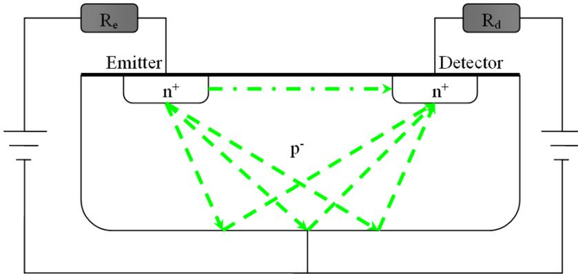
**Figure 2.14:** Test setup for optical crosstalk evaluation. Light generated in an avalanche, can travel with or without reflections through the substrate [59].
