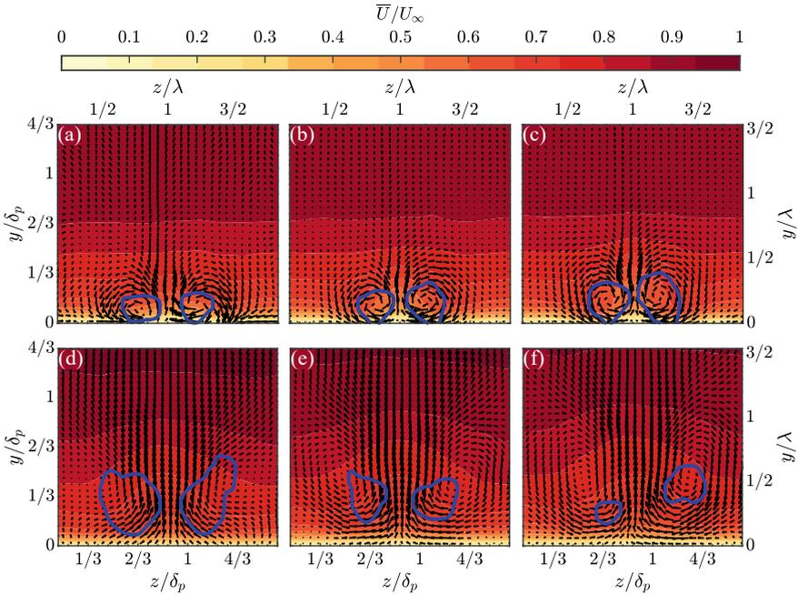
**Fig. 2** Evolution of plasma actuation in the  $y-z$  plane at  $\hat{x} = \delta_p$  (a),  $3\delta_p$  (b),  $5\delta_p$  (c),  $14\delta_p$  (d),  $16\delta_p$  (e),  $18\delta_p$  (f). The contour depicts the streamwise velocity distribution at each plane. The quiver represents the flow motion based on  $\bar{V}$  and  $\bar{W}$  velocity components. Negative  $\lambda_2$  isolines (—) illustrate the locations of vortical flow structures
