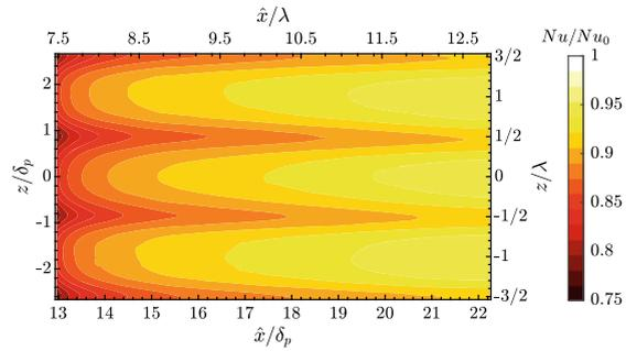
over the whole region where the actuator array is deployed, and a localized, predominant decrease at the location where the plasma plumes lift-off to promote out-of-the-wall motion. Eventually, the plasma forcing provides a reduction of 9% in convective heat transfer within the region covered by the heat-flux sensor, far downstream the DBD-plasma actuator.
