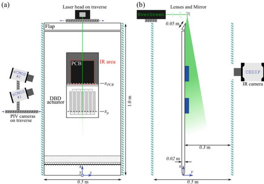
**Fig. 1** Schematic of the experimental setup. **a** Front view; the measurement area of infrared thermography is indicated (---). **b** Side view; the field of views of the stereo-PIV measurements are highlighted (■)
