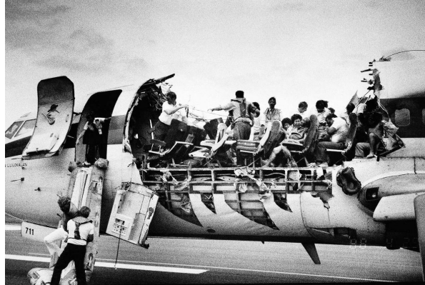
Figure 1.2: The Aloha flight 243 damage after an explosive decompression and structural failure during cruise flight [14].
