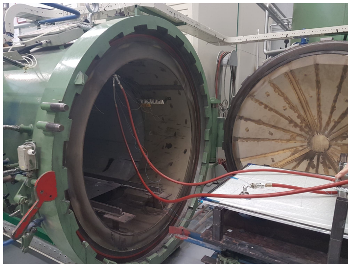
Figure 4.4: The autoclave used for part consolidation, with controlled temperature (T) and pressure (P).
