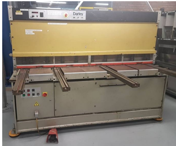
Figure 4.2: The Darley machine used for cutting the aluminum into the desired shape and dimensions.
