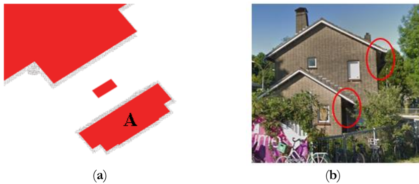
Figure 5.13 Comparison of Bag building polygon (red) and the AHN3 building points (grey) in case of overhanging roof. (a) Top view building definition of BAG polygon (red) and the AHN3 building points (grey); (b) Building “A” has overhanging roof (red circle) ©GoogleStreetView.
