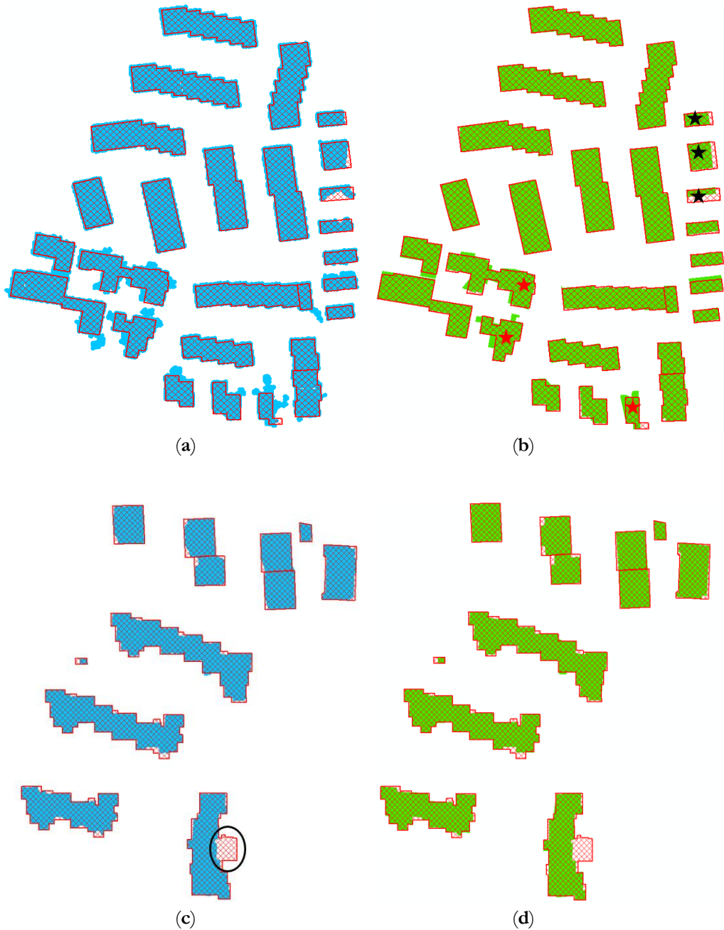
Figure 4.17 Comparison of building outline results with ground truth. (a–b) Vaihingen-A test area; (c–d) Vaihingen-B test area. Left: comparison of filtered building points (blue) and base map (red polygons); Right: outlines generated by the proposed method (green) and base map (red polygons).
