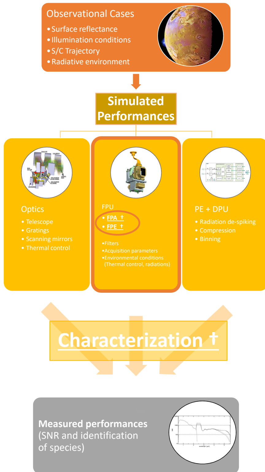
Figure 1.1: Overview of the elements contributing to the SNR of the MAJIS instrument
