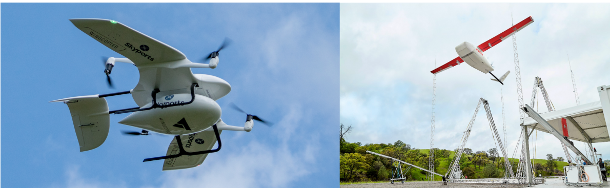
Figure 1.1: Drones performing aerial delivery of medical supplies; A hybrid tilt rotor UAV (left) and a fixed wing delivery drone (right)
