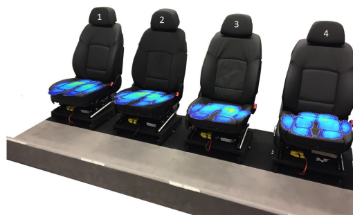
Figure 8.4: Comparison of the results of the pressure mat measurements related to the case study presented in chapter 7. From left to right: reference seat / original BMW 5-series seat (seat 1); Alcantara seat (seat 2); loose cover tension (seat 3), and seat with a metal plate instead of a seat suspension (seat 4).
