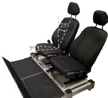
Figure 4.1: Setup of the experiment. Leather and fabric seat mounted next to each other in the H-Point-Position.
