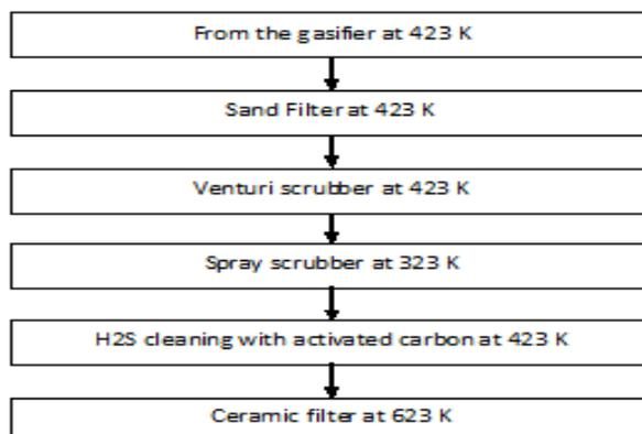
Figure 1. Flow scheme for the tested low temperature gas-cleaning system.
