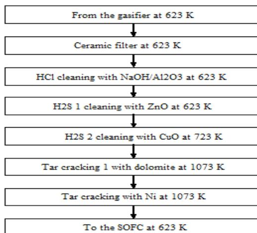
Figure 3. Flow scheme for the intermediate temperature gas-cleaning system.
