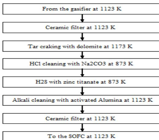
Figure 2. Flow scheme for the high temperature gas-cleaning system.
